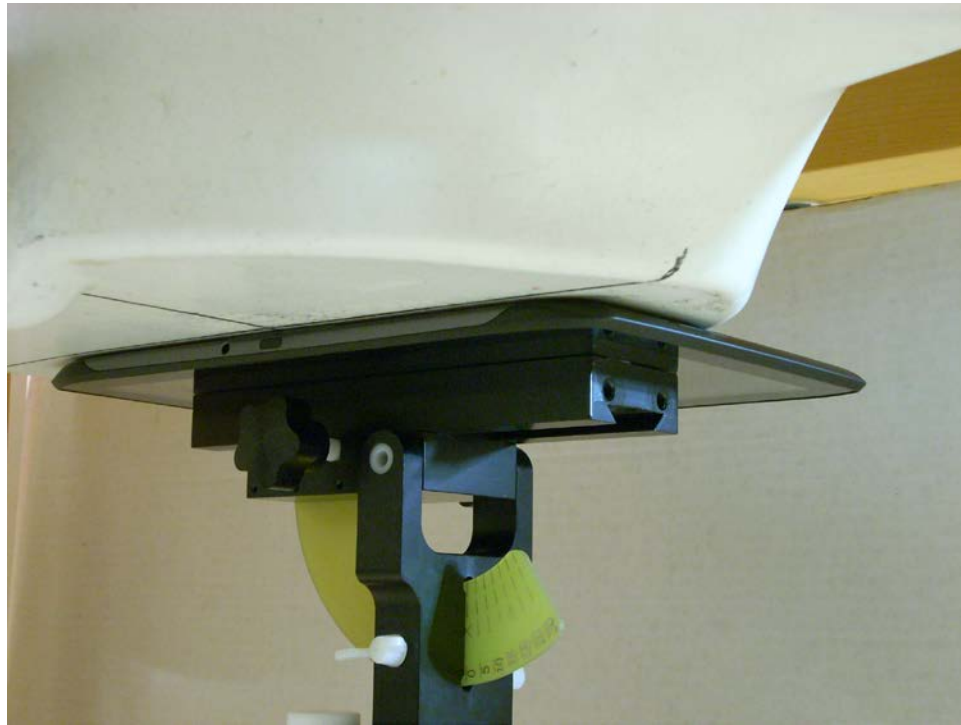
SAR Test Setup Photo 1 - Back at 0.0 cm
