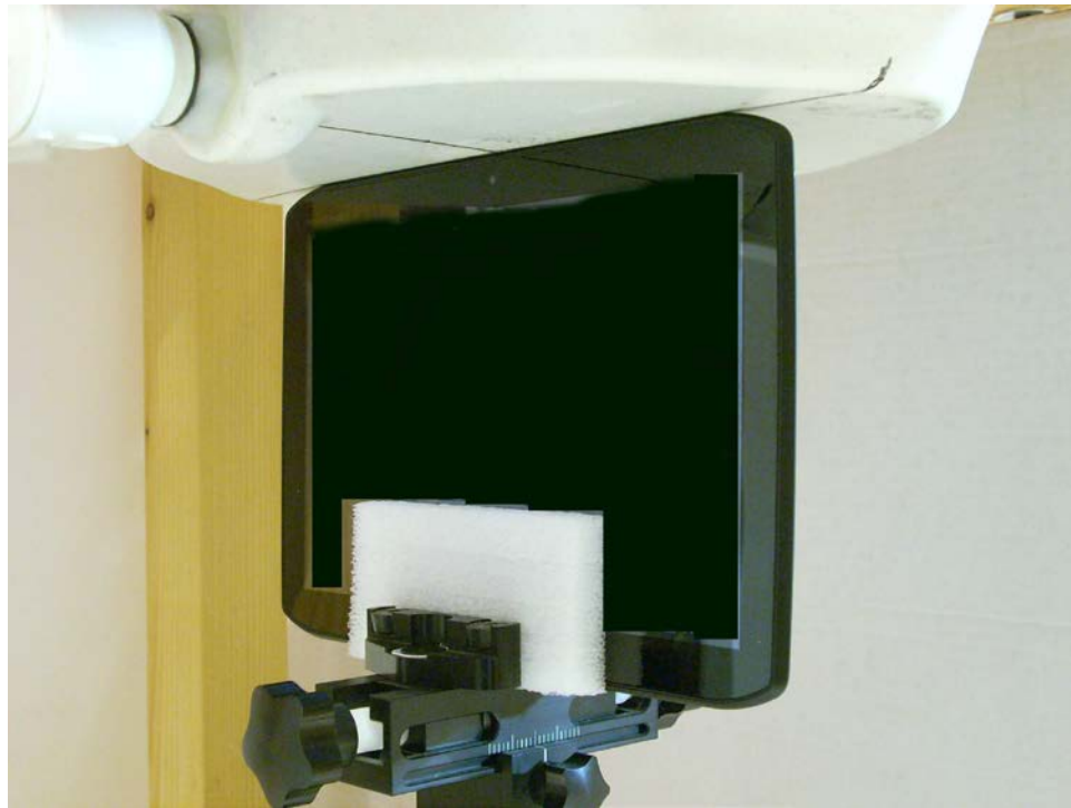
SAR Test Setup Photo 2 – Top at 0.0 cm
