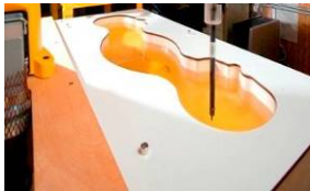
Figure 6-2 SAM Phantom with Simulating Tissue
