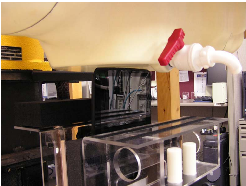
Figure 6: Right Edge of DUT toward Phantom, 0 mm Separation
