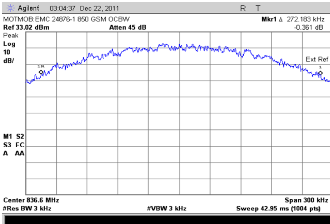
GSM 850 – Channel 190 (836.60 MHz) – Occupied Bandwidth
