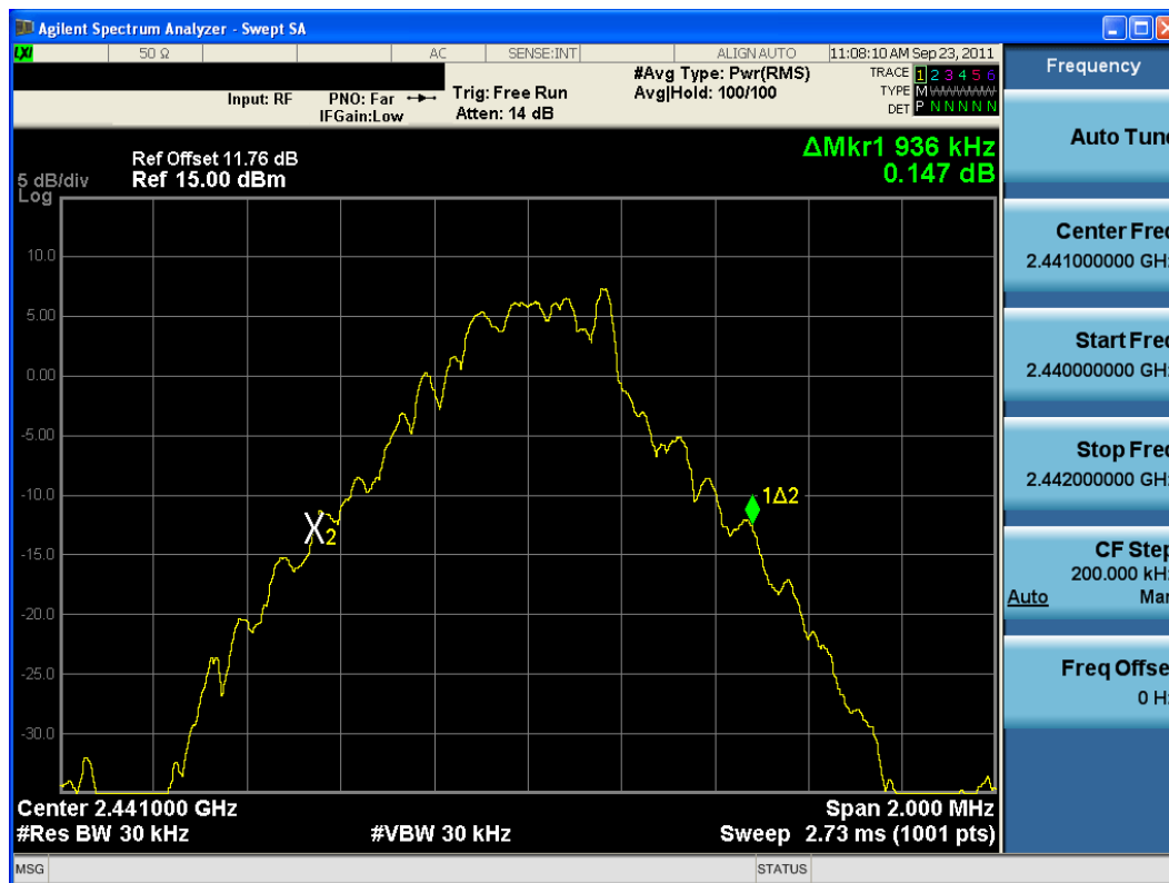
Plot 6-2. 20dB Bandwidth Plot (Bluetooth, 1Mbps – Ch. 39)
