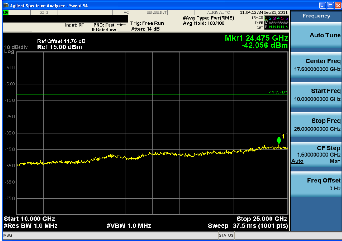
Plot 6-21. Conducted Spurious Plot (Bluetooth, 3Mbps – Ch. 0)
