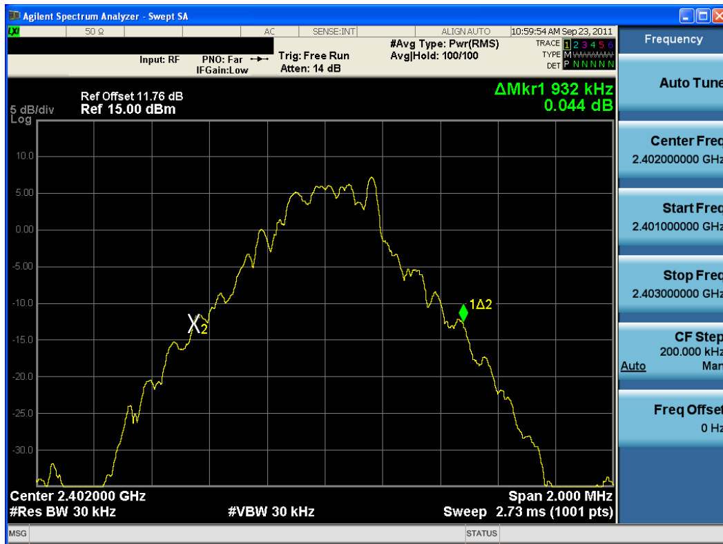
Plot 6-1. 20dB Bandwidth Plot (Bluetooth, 1Mbps – Ch. 0)
