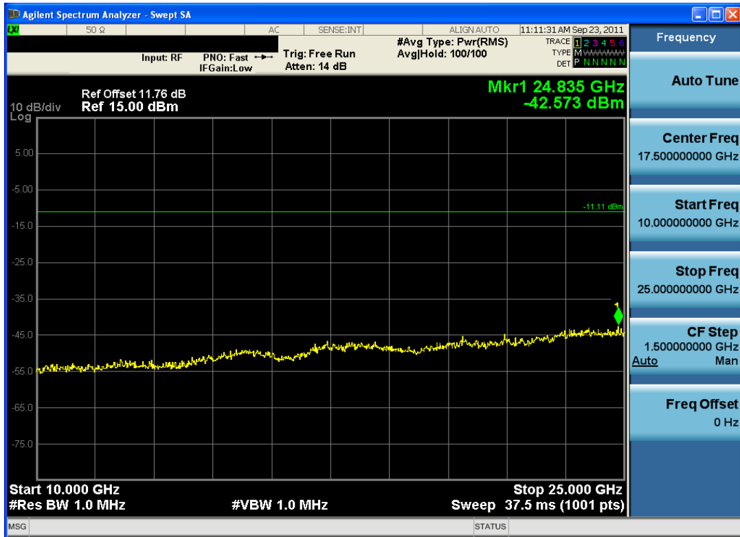
Plot 6-25. Conducted Spurious Plot (Bluetooth, 3Mbps – Ch. 78)
