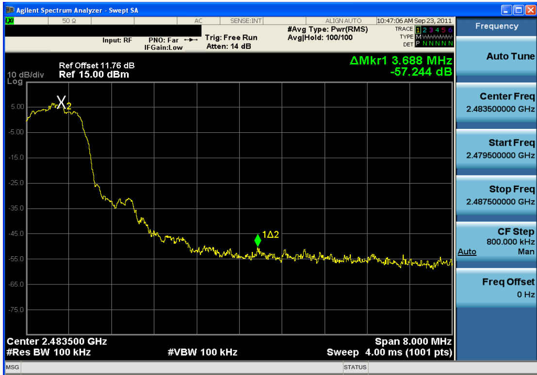
Plot 6-14. Band Edge Plot (Bluetooth, 3Mbps – Ch. 78)
