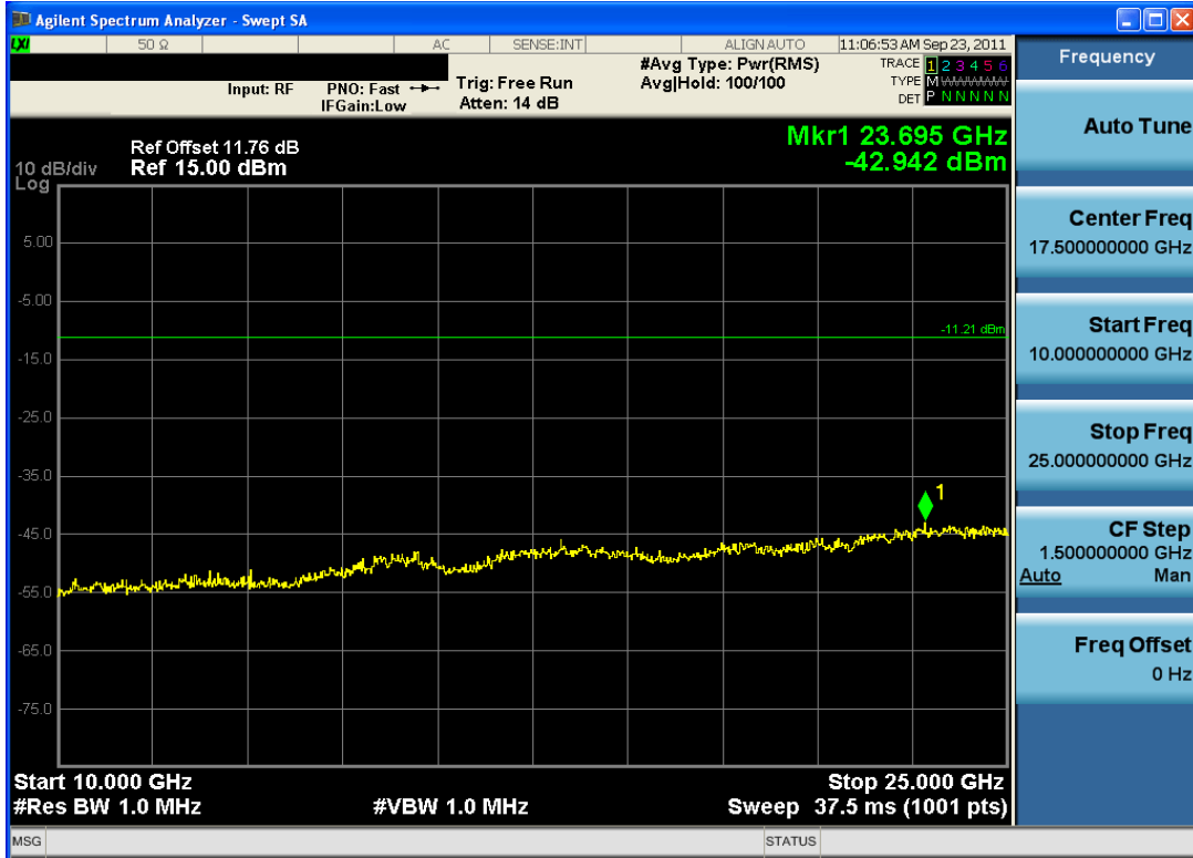
Plot 6-23. Conducted Spurious Plot (Bluetooth, 3Mbps – Ch. 39)
