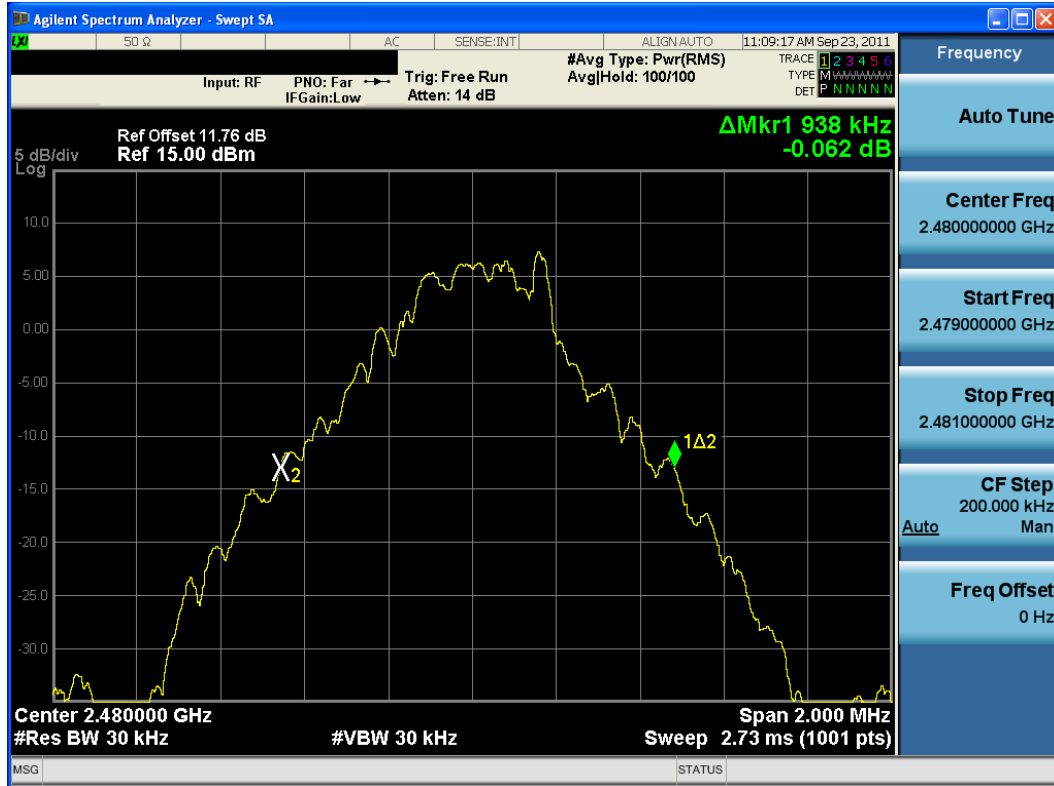
Plot 6-3. 20dB Bandwidth Plot (Bluetooth, 1Mbps – Ch. 78)
