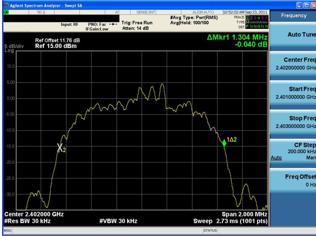
Plot 6-7. 20dB Bandwidth Plot (Bluetooth, 3Mbps – Ch. 0)
