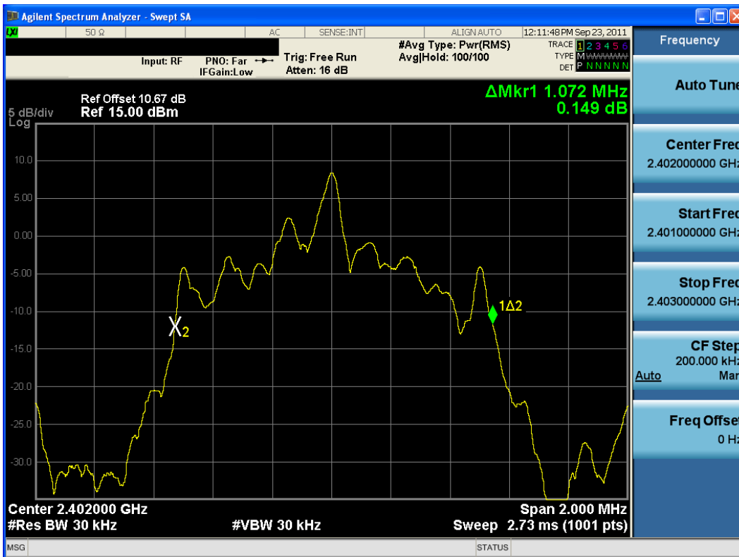
Plot 6-10. 20dB Bandwidth Plot (Bluetooth LE Mode – Ch. 0)
