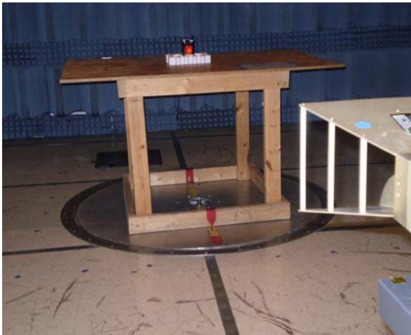
Figure 4: Transmitter Spurious Emissions Test Set-up.
