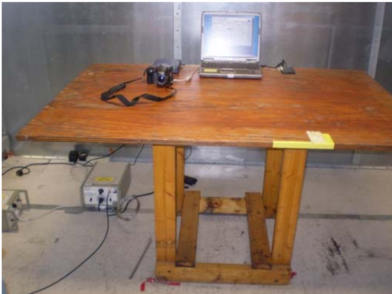
Figure 1: Part 15 AC Line Spurious Voltages Test Set-up.
