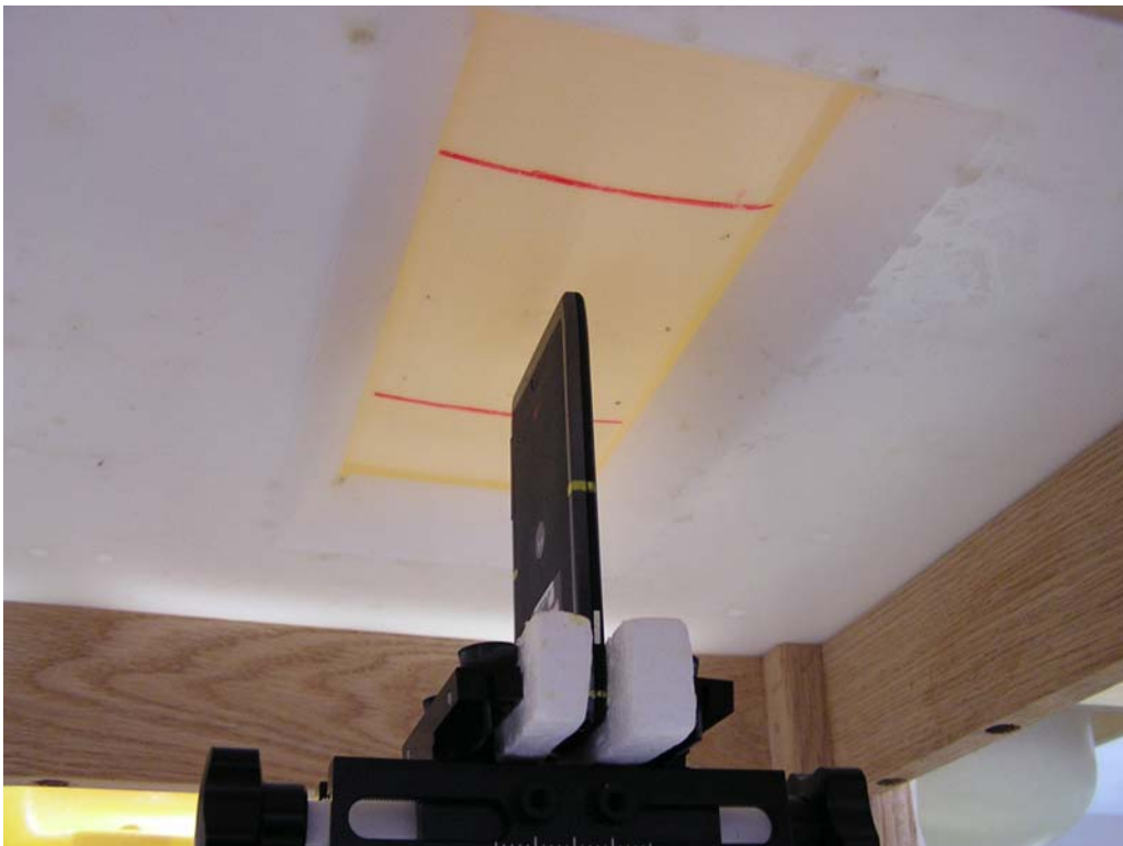
Figure 10: Mobile Hotspot Position, Bottom Edge of Phone facing Phantom (10 mm separation)
