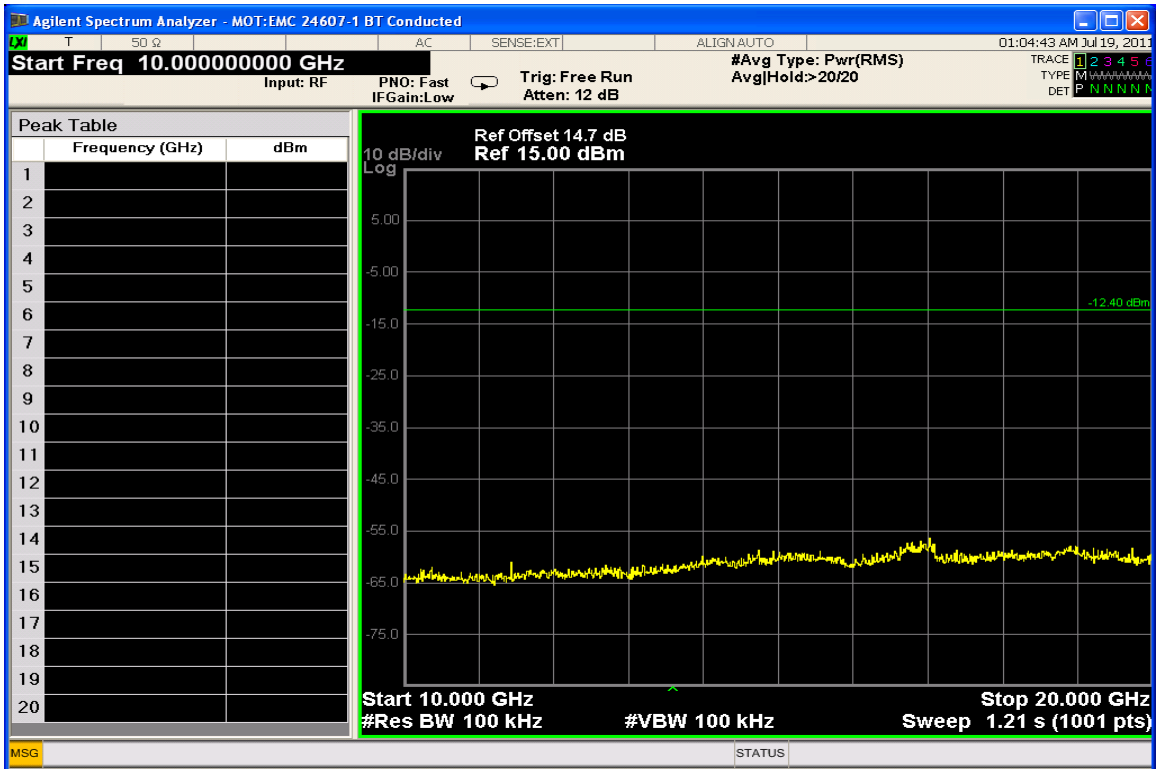
Conducted Spurious Emissions 10-20GHz (Low Channel Enabled)
