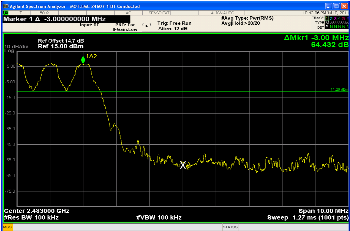
High Band edge with Hopping Enabled
