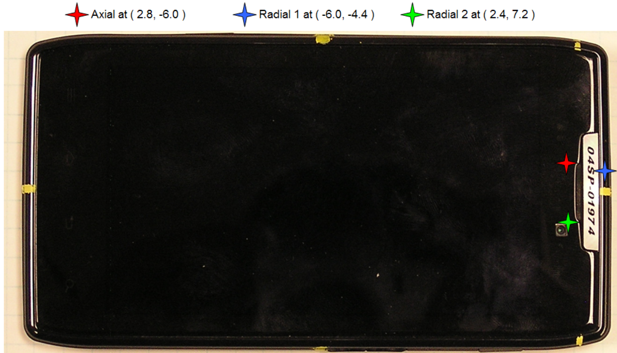
Figure 5. Location of point measurements for ABM (Telecoil) Emissions
