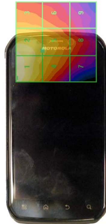
Figure 17-5 H-Field WD Scan overlay
