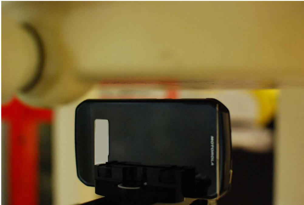
Figure 22-8 SAR Test Setup Photo – Left at 1.0 cm
