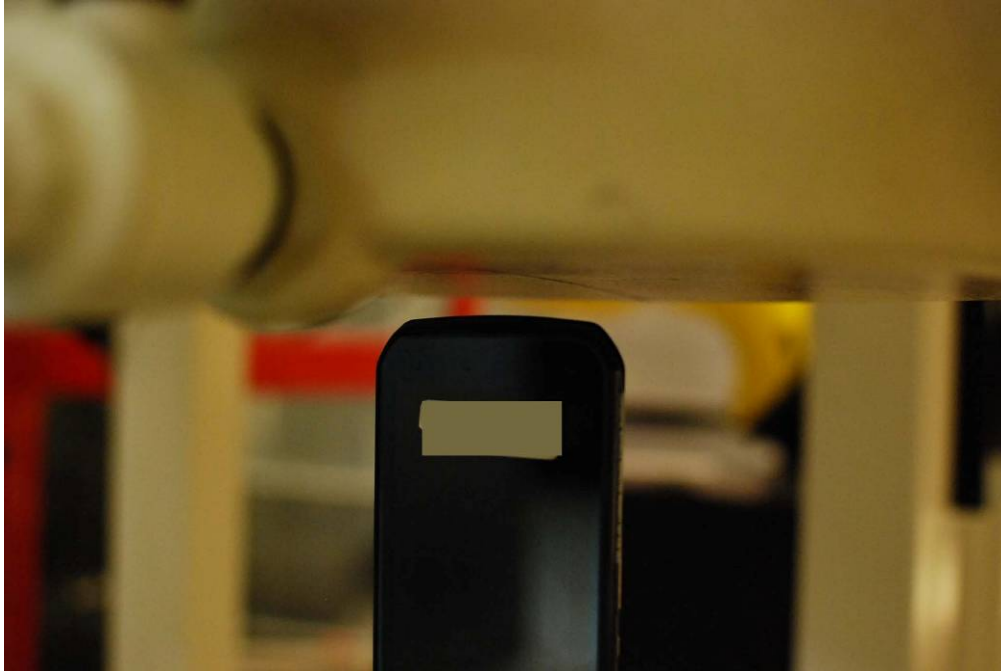
Figure 22-7 SAR Test Setup Photo – Bottom at 1.0 cm
