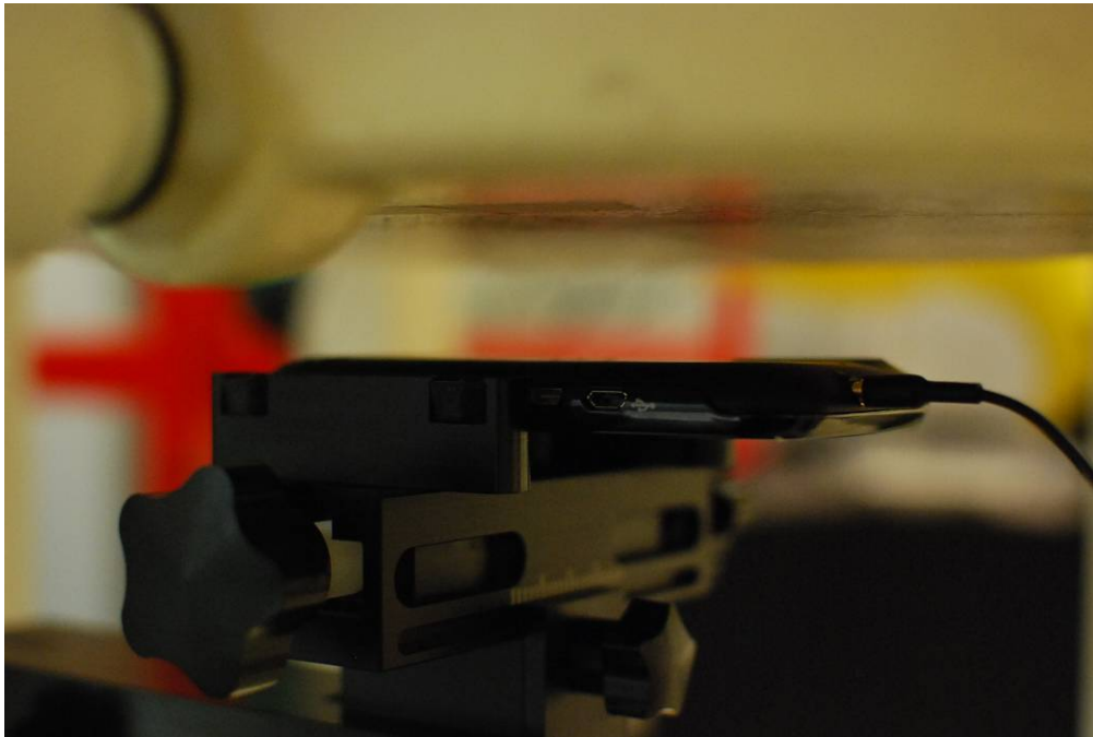
Figure 22-10 SAR Test Setup Photo – Body-Worn at 2.5 cm
