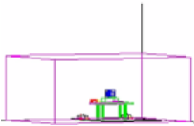
Figure 3-1. Shielded Enclosure Line-Conducted Test Facility
