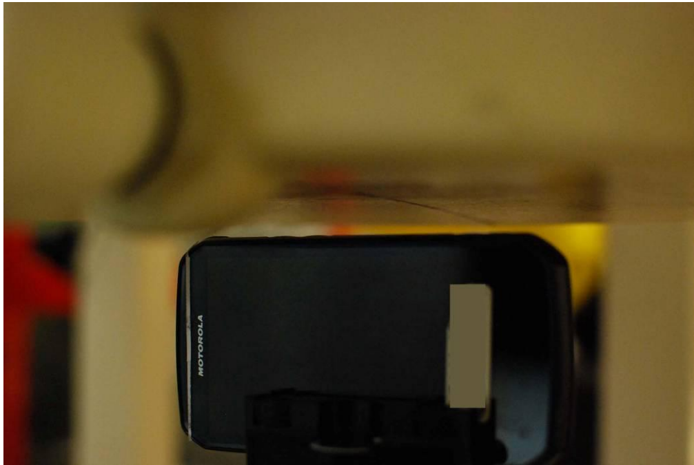
Figure 24-10 SAR Test Setup Photo – Right at 1.0 cm
