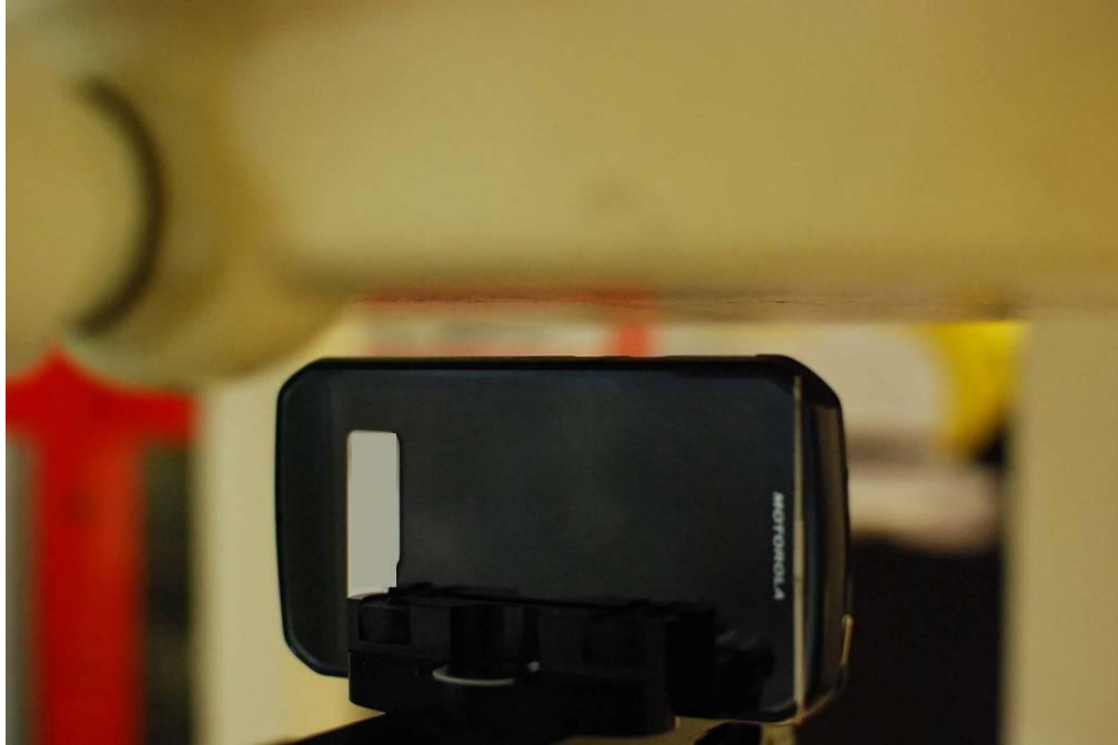
Figure 24-9 SAR Test Setup Photo – Left at 1.0 cm
