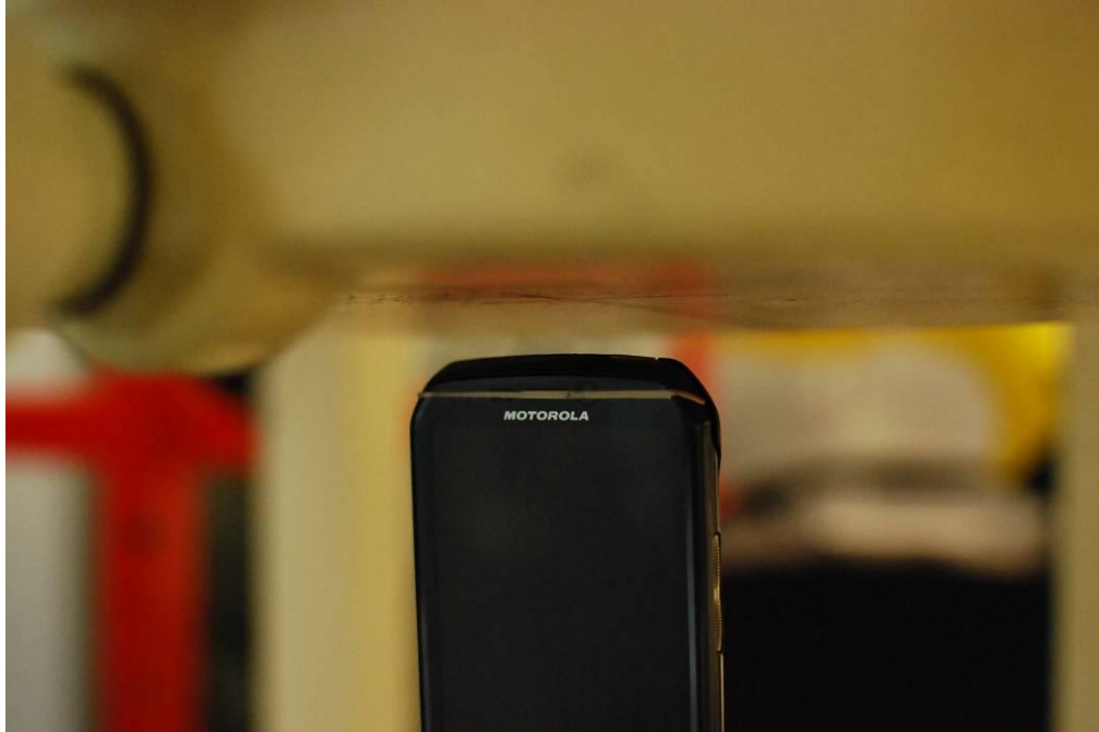
Figure 24-7 SAR Test Setup Photo – Top at 1.0 cm
