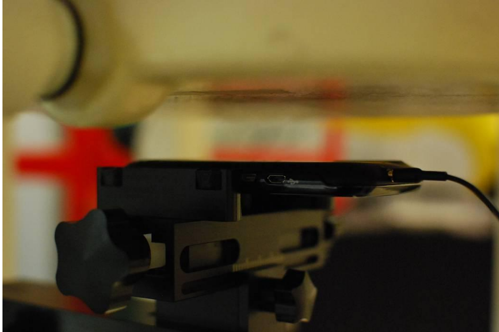
Figure 24-11 SAR Test Setup Photo – Body-Worn at 2.5 cm
