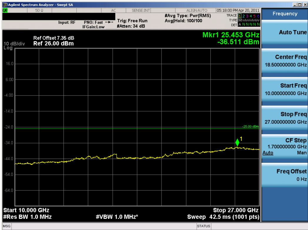
Plot 8-32. Conducted Spurious Plot (High Ch., 10MHz BW, QPSK, Antenna 1)
