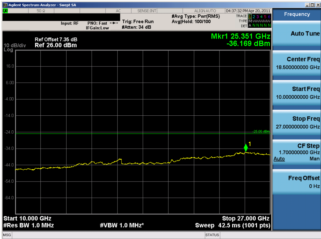
Plot 8-38. Conducted Spurious Plot (High Ch., 10MHz BW, QPSK, Antenna 2)
