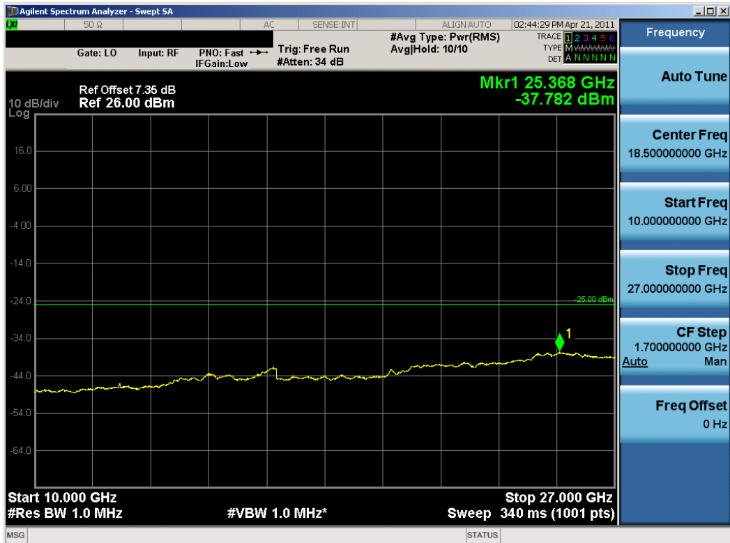
Plot 7-4. Conducted Spurious Plot (Low Ch., 5MHz BW, QPSK, Antenna 1)
