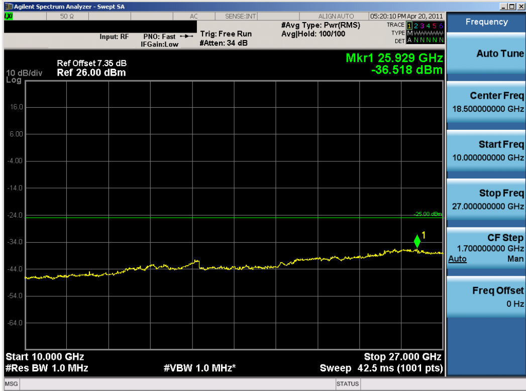
Plot 8-17. Conducted Spurious Plot (Mid Ch., 10MHz BW, QPSK Antenna 1)
