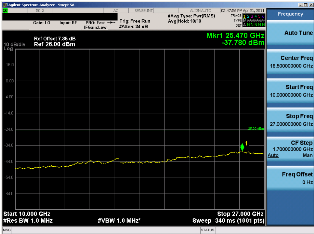
Plot 7-10. Conducted Spurious Plot (Low Ch., 5MHz BW, QPSK, Antenna 2)
