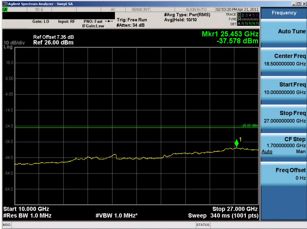
Plot 7-17. Conducted Spurious Plot (Mid Ch., 5MHz BW, QPSK Antenna 1)
