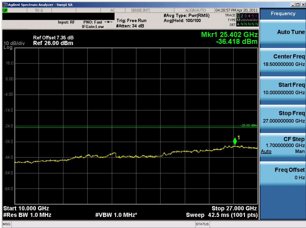
Plot 8-10. Conducted Spurious Plot (Low Ch., 10MHz BW, QPSK, Antenna 2)
