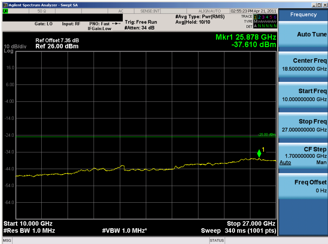
Plot 7-32. Conducted Spurious Plot (High Ch., 5MHz BW, QPSK, Antenna 1)
