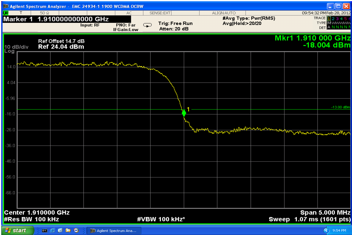
WCDMA 1900 – Upper Band Edge – Channel 9538 (1907.60 MHz)
