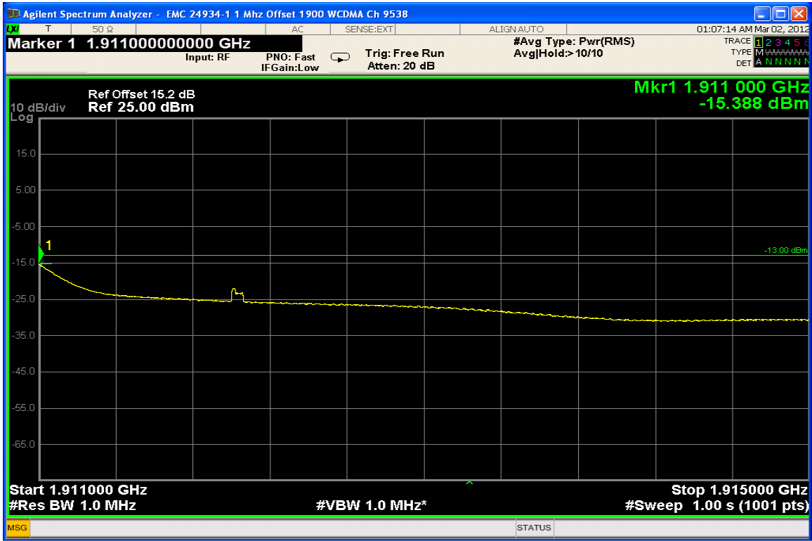
1900 WCDMA Conducted Spurious Emissions (Upper adjacent 1 MHz band)
