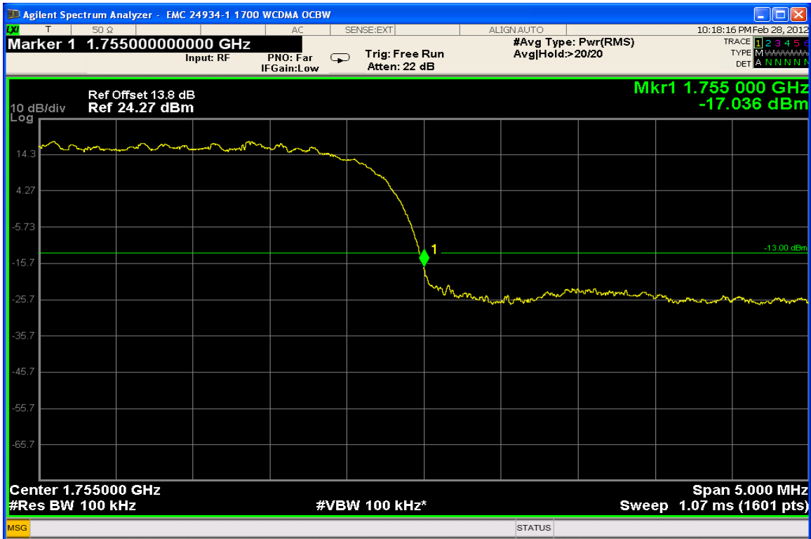
WCDMA 1700 – Upper Band Edge – Channel 1513 (1752.6 MHz)
