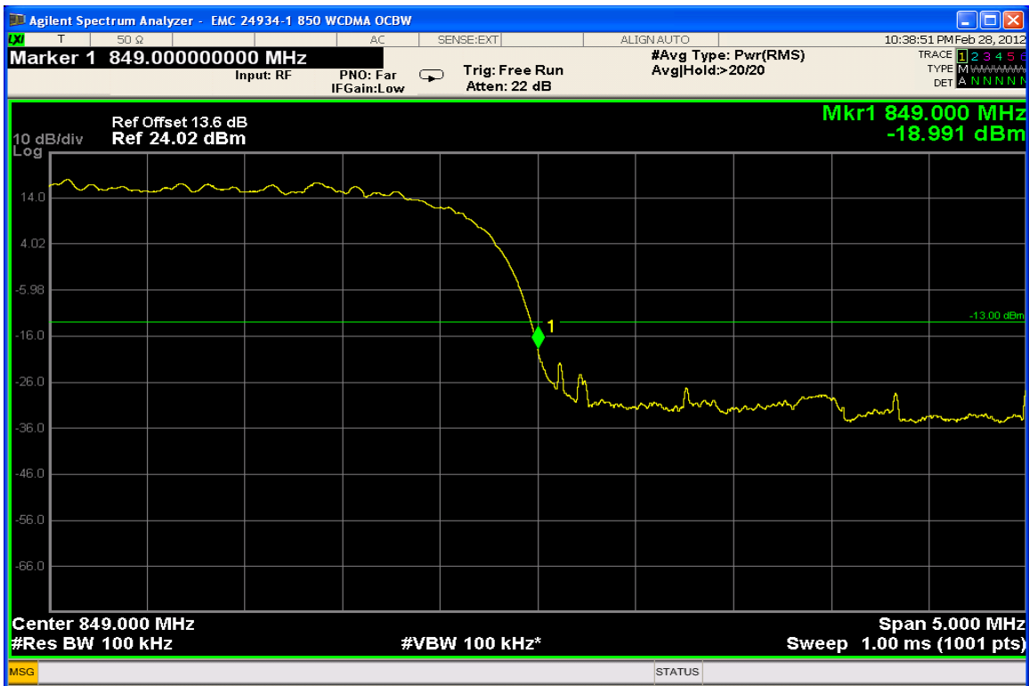
WCDMA 850 – Upper Band Edge – Channel 4233 (846.6 MHz)
