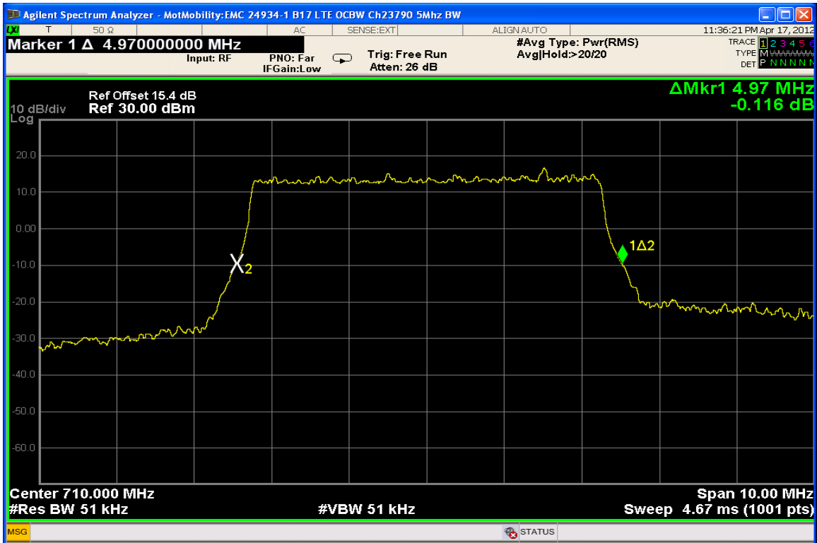
Band 17 LTE - 5MHz BW, QPSK RB Size = 25 RB Start 0
