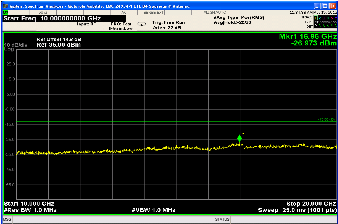
5MHz BW, QPSK RB Size = 25RB Start 0, High Channel
