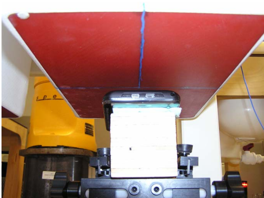
Figure 5: Body Position (25 mm separation)
