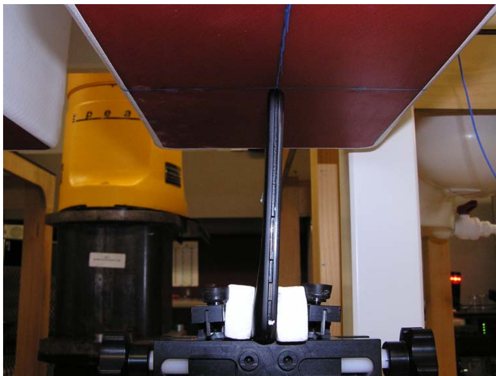
Figure Figure 8: Mobile Hotspot Position, Shot Edge (Bottom / Top) of Phone facing Phantom (10 mm separation)
