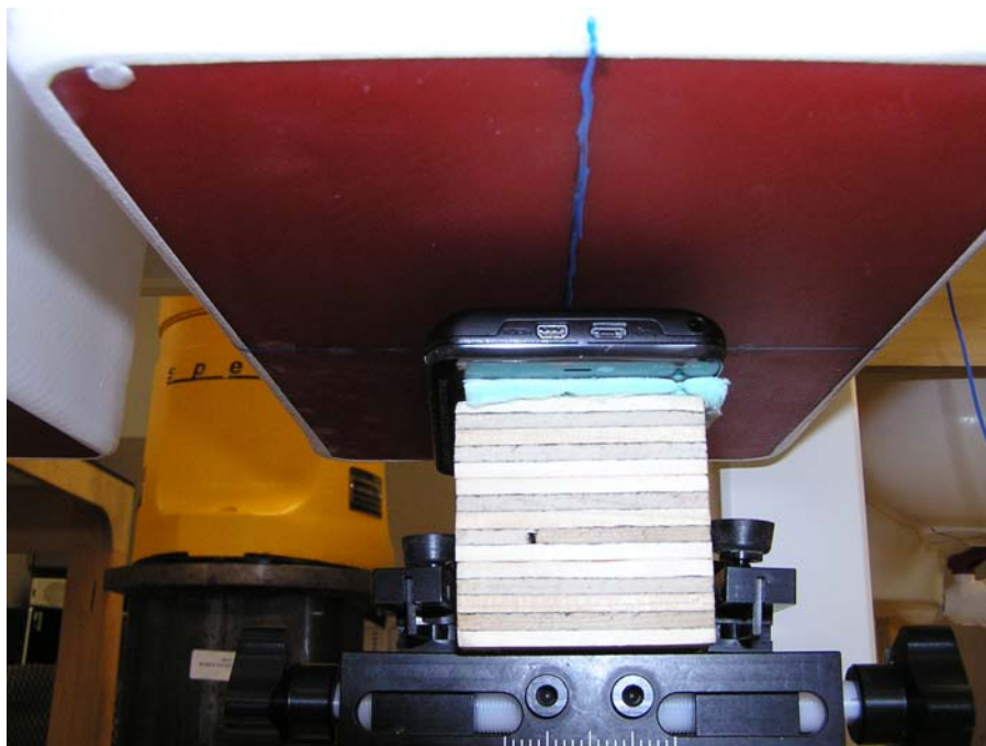
Figure 6: Mobile Hotspot Position, Back of Phone facing Phantom (10 mm separation)
