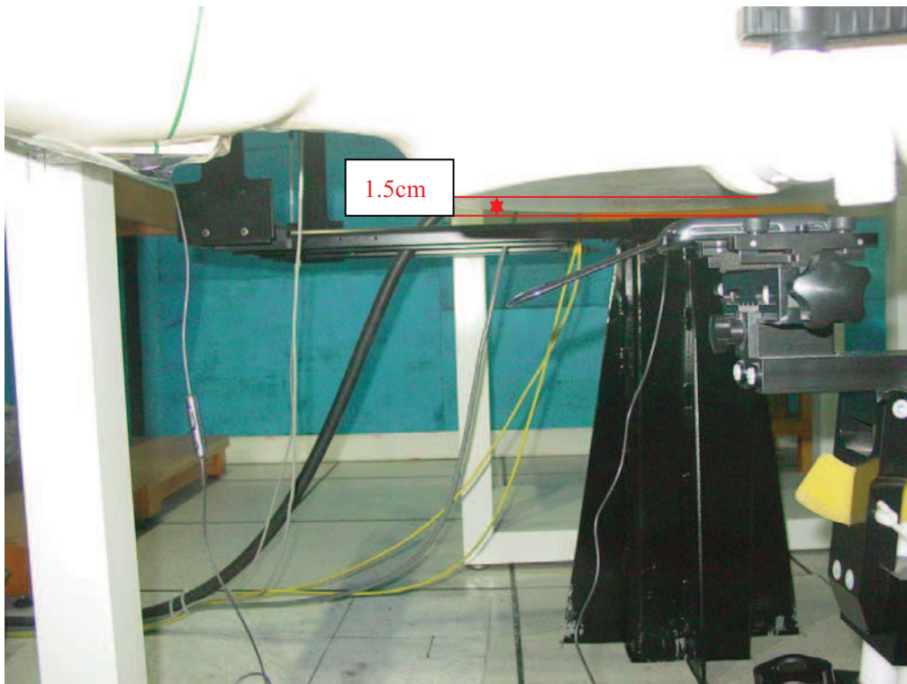
Picture B12: Body-worn Position with Headset (towards ground, the distance from handset to the bottom of the Phantom is 1.5cm)
