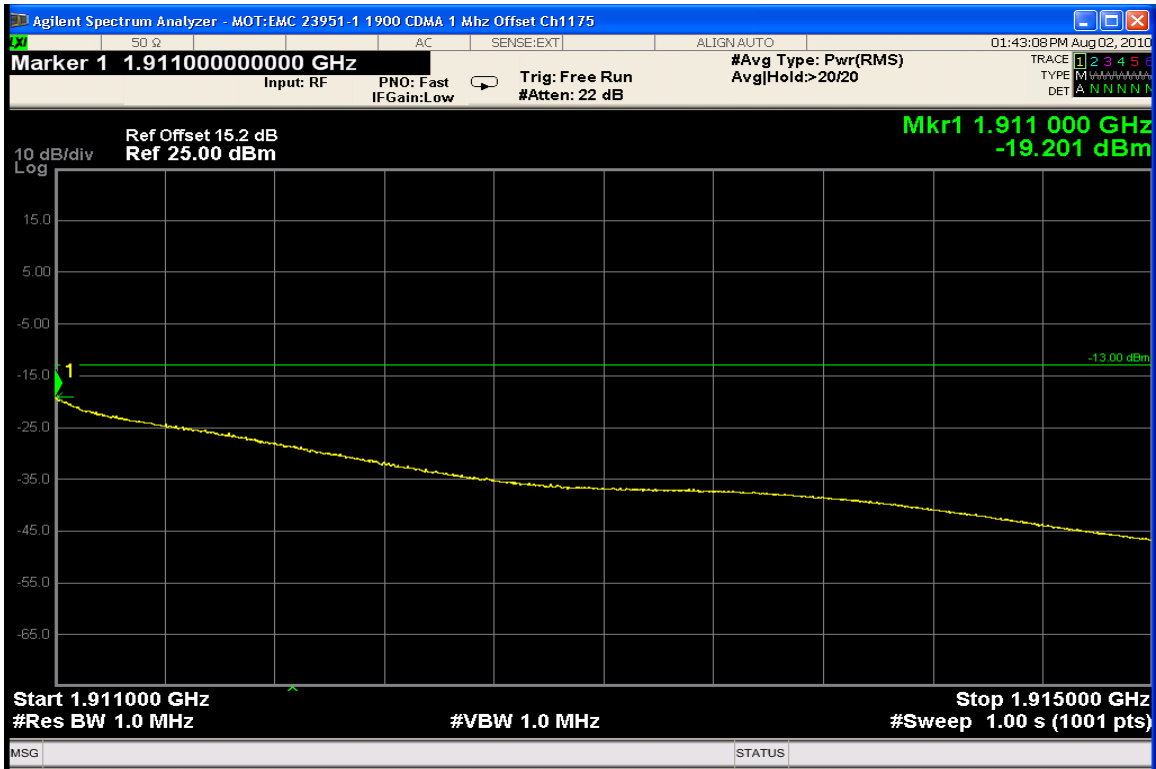
PCS Conducted Spurious Emissions (Upper adjacent 1 MHz band)
