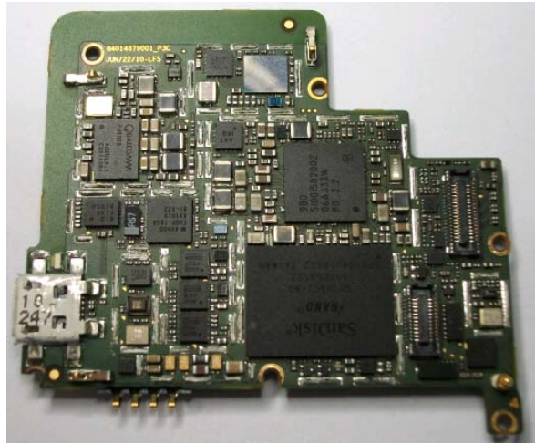
Front of Main PCB without Shield Can
