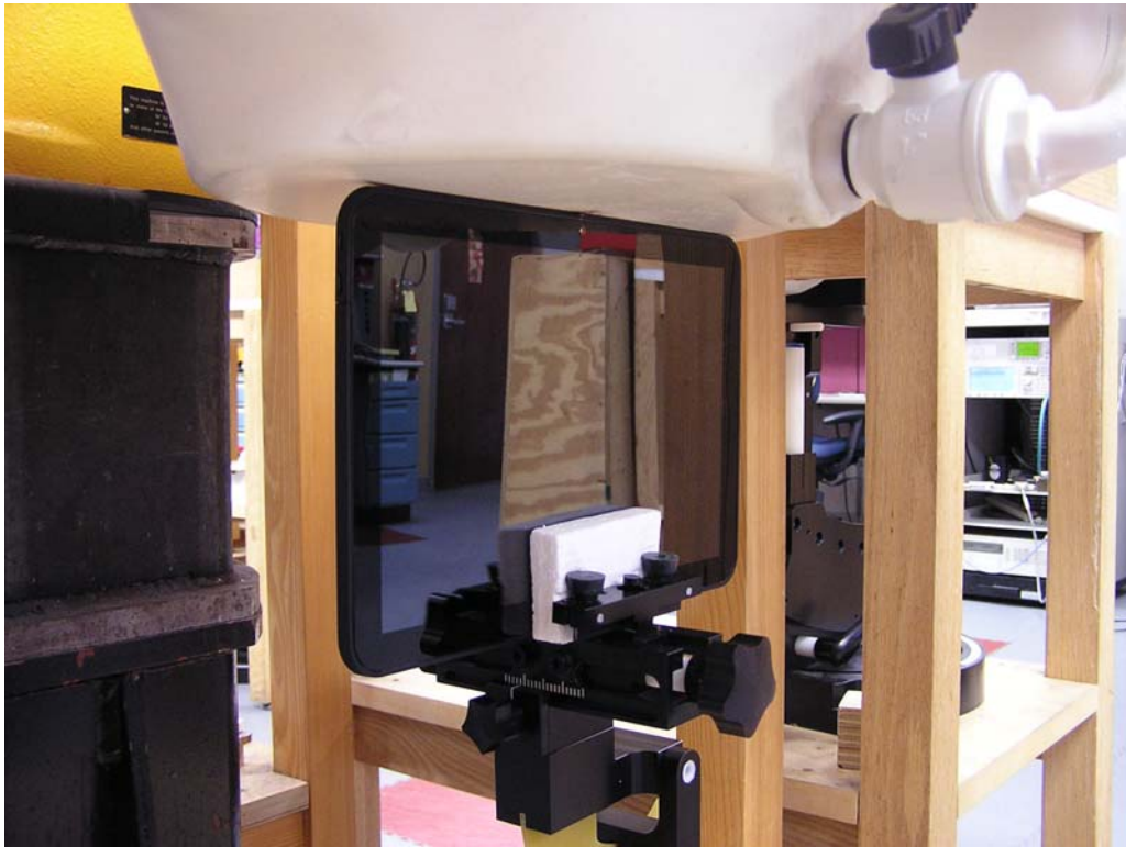
Figure 7: Top Edge of Host Device and DUT toward Phantom, 0 mm Separation
