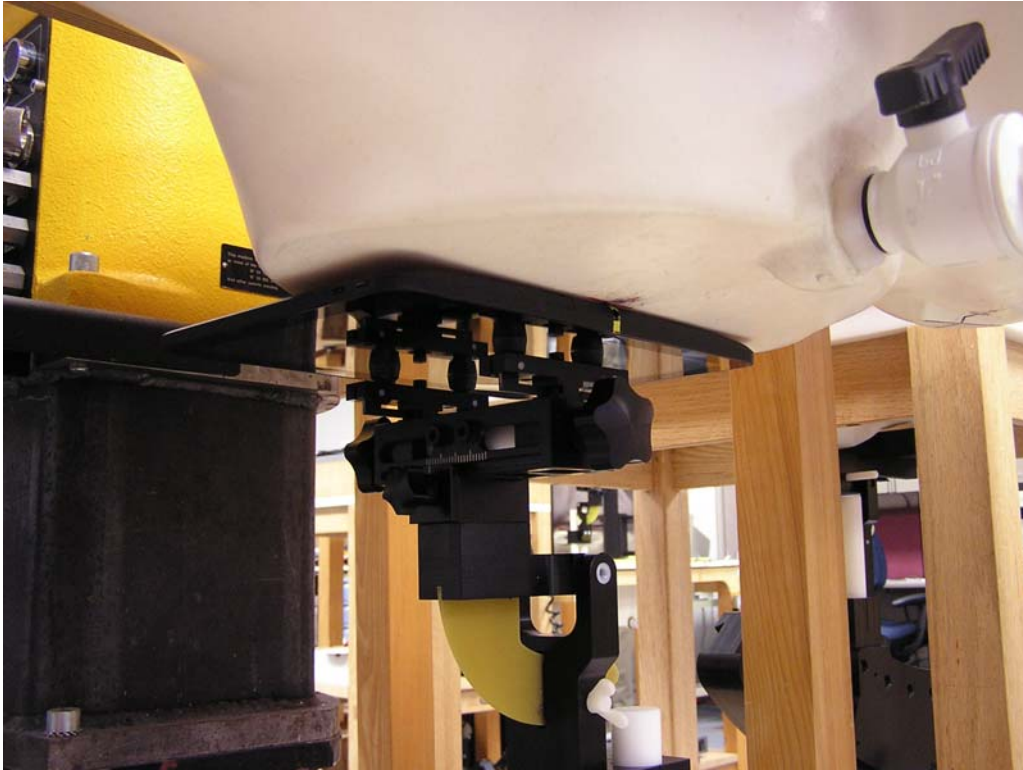
Figure 6: Back Surface of Host Device & DUT toward Phantom, 0 mm Separation
