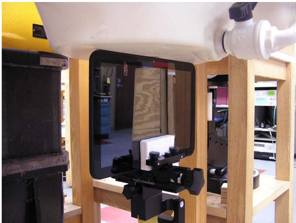
Figure 5: Top Edge of DUT toward Phantom, 0 mm Separation
