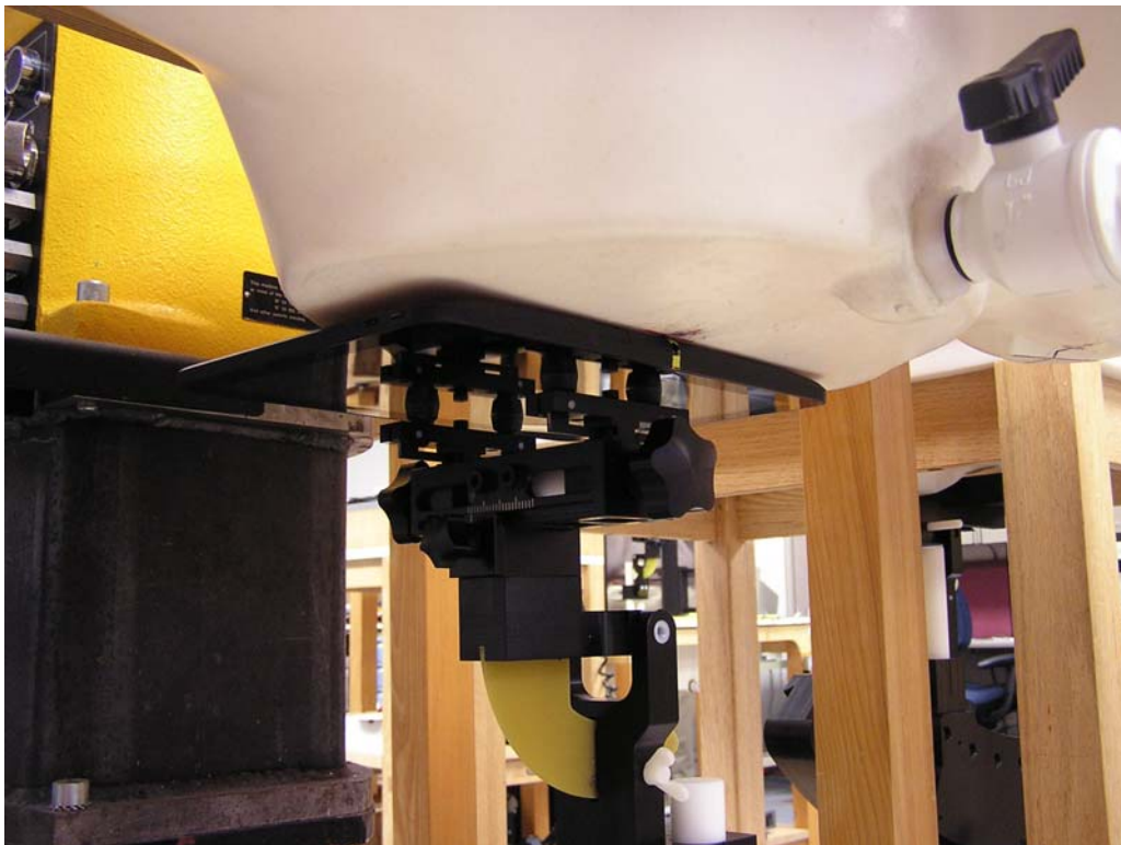
Figure 4: Back Surface of DUT toward Phantom, 0 mm Separation
