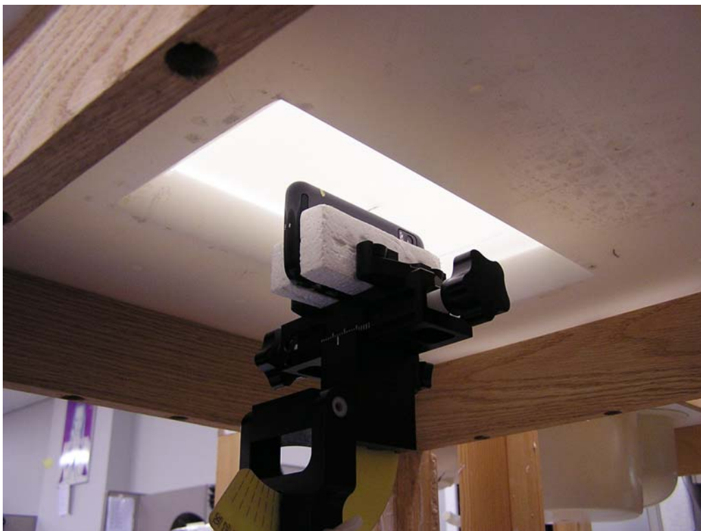
Figure 9: Mobile Hotspot Position, Right Edge of Phone facing Phantom (10 mm separation)
