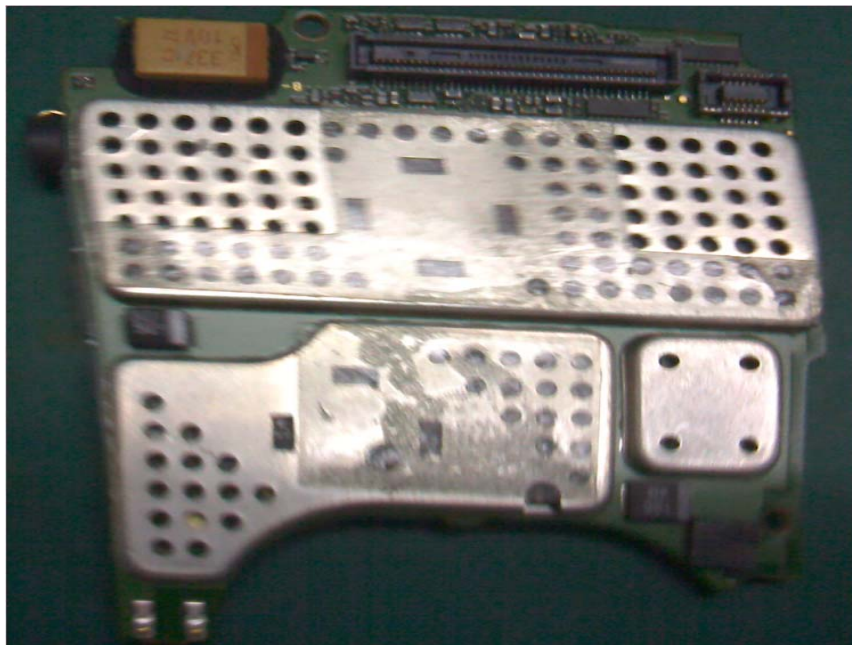
Photograph 9-1: Front side view of radio product PC Board; shields in place.
