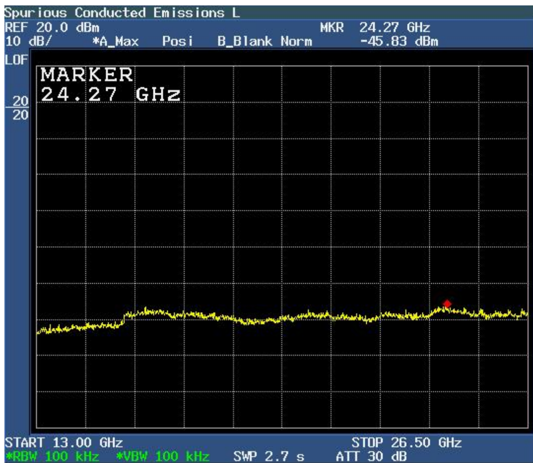
Figure 6c.8-3: Plot of spurious conducted emissions 13 GHz – 26.5 GHz (Low Channel Enabled).
