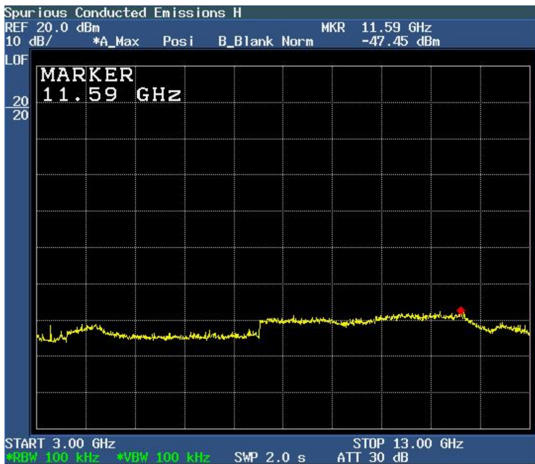
Figure 6c.8-8: Plot of spurious conducted emissions 3 GHz – 13 GHz (High Channel Enabled).
