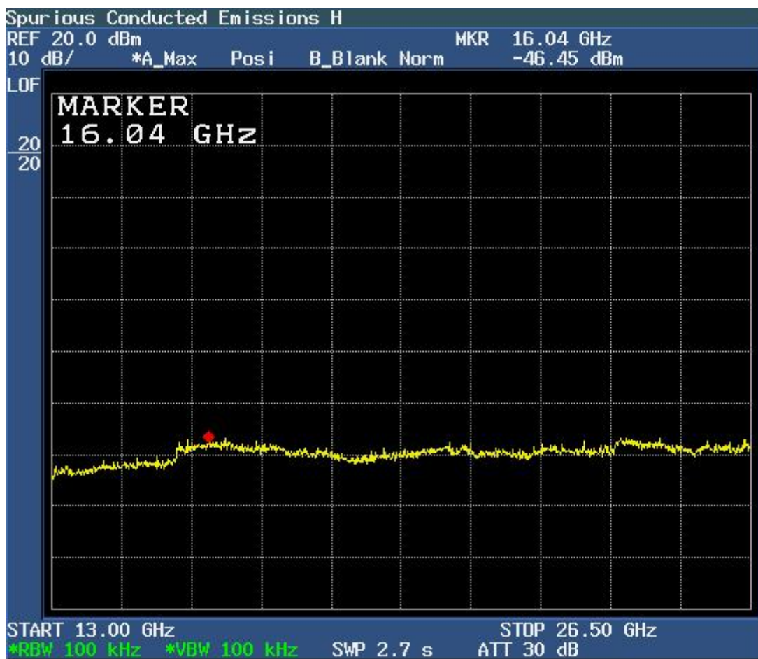
Figure 6c.8-9: Plot of spurious conducted emissions 13 GHz – 26.5 GHz (High Channel Enabled).
