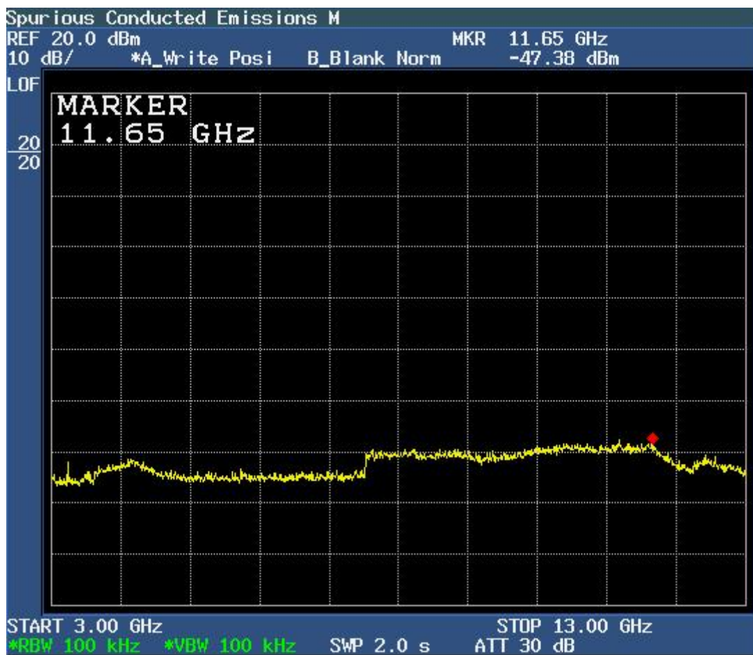
Figure 6c.8-5: Plot of spurious conducted emissions 3 GHz – 13 GHz (Mid Channel Enabled).
