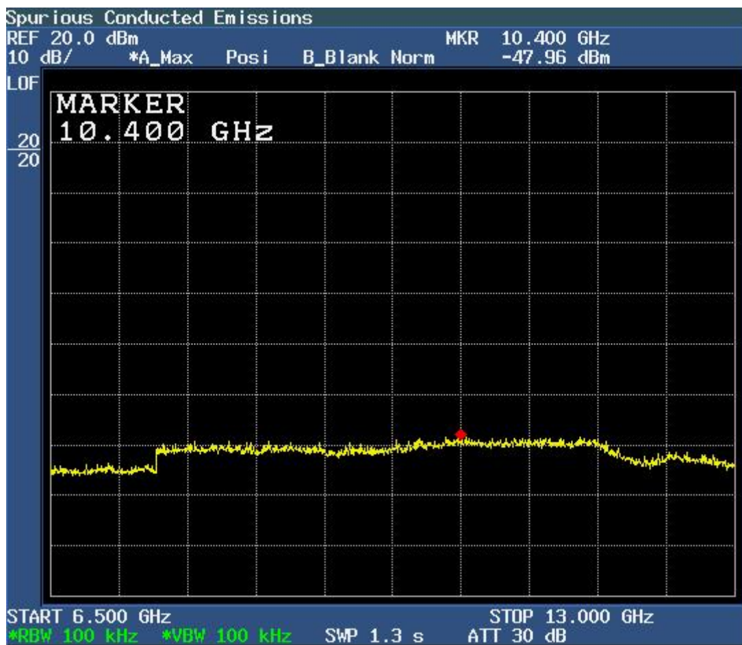
Figure 6c.8-12: Plot of spurious conducted emissions 6.5 GHz – 13.0 GHz (Hopping Enabled).
