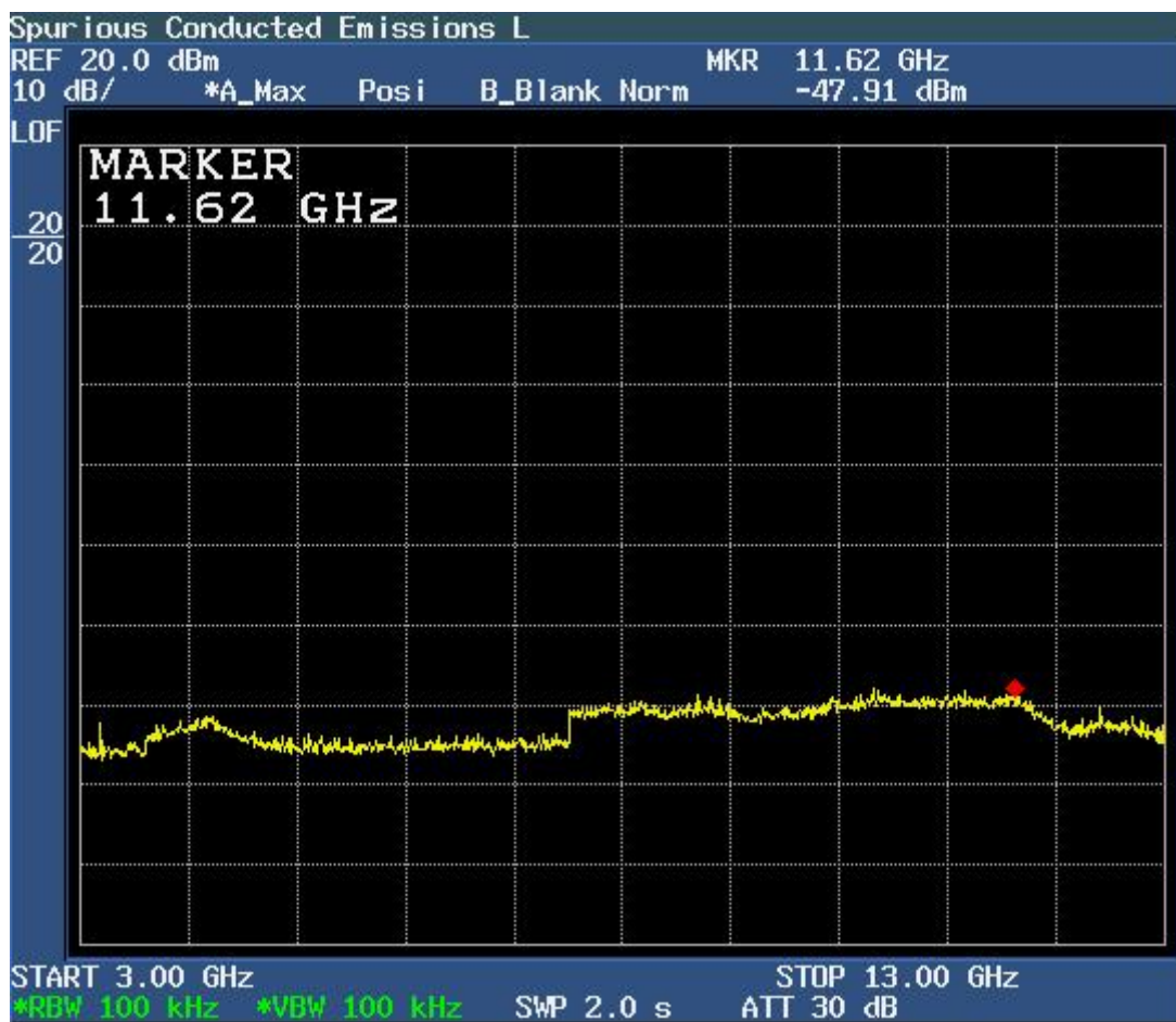
Figure 6c.8-2: Plot of spurious conducted emissions 3 GHz – 13 GHz (Low Channel Enabled).
