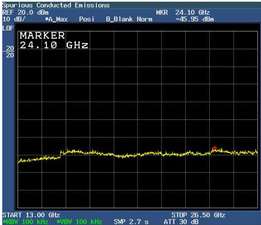
Figure 6c.8-13: Plot of spurious conducted emissions 13.0 GHz – 26.5 GHz (Hopping Enabled).
