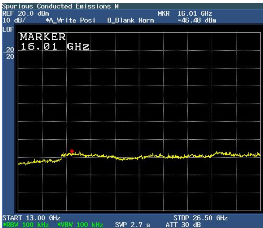
Figure 6c.8-6: Plot of spurious conducted emissions 13 GHz – 26.5 GHz (Mid Channel Enabled).
