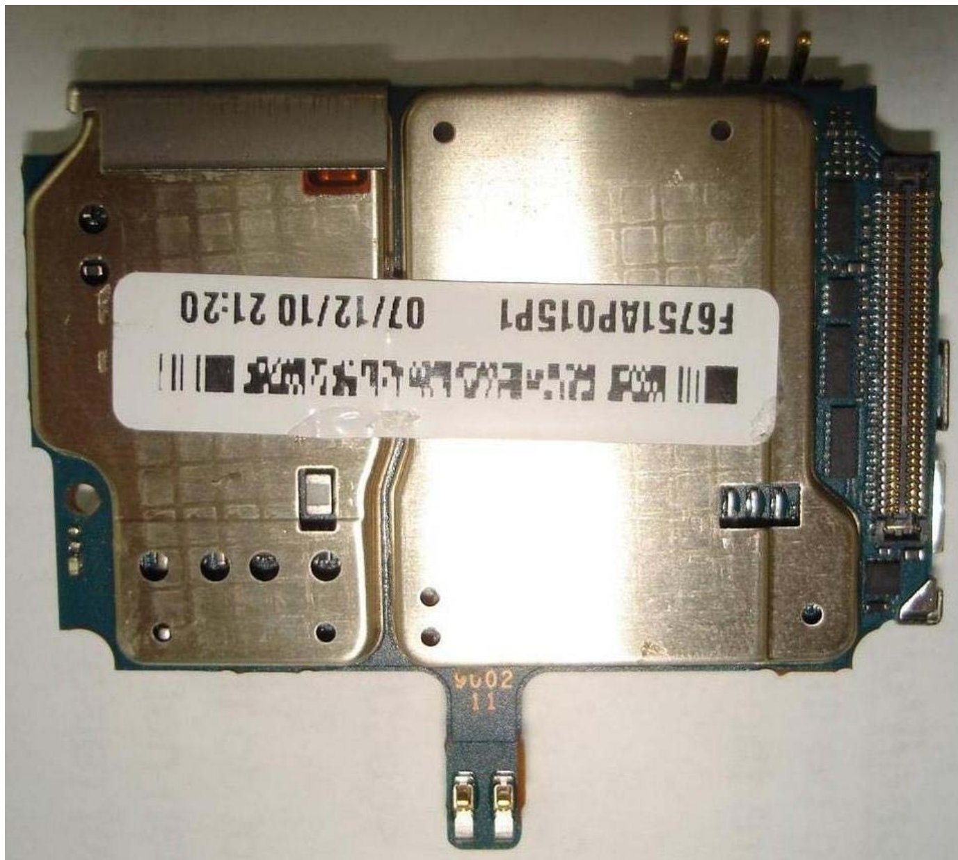
Photograph 9-1: Front side view of radio product PC Board, Shields in Place.
