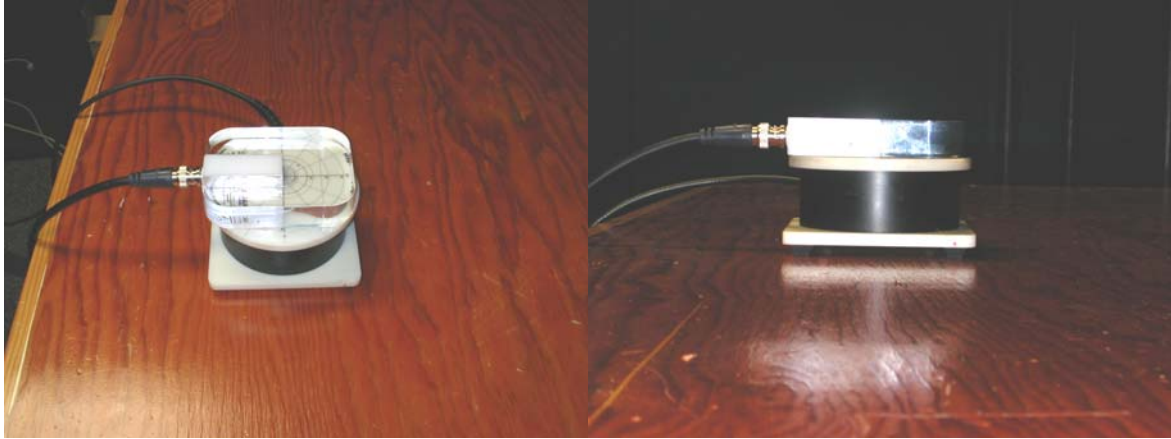
Figure 6-1 – Probe coil being calibrated with TMFS
