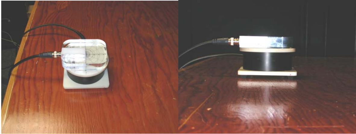
Figure 6-1 – Probe coil being calibrated with TMFS
