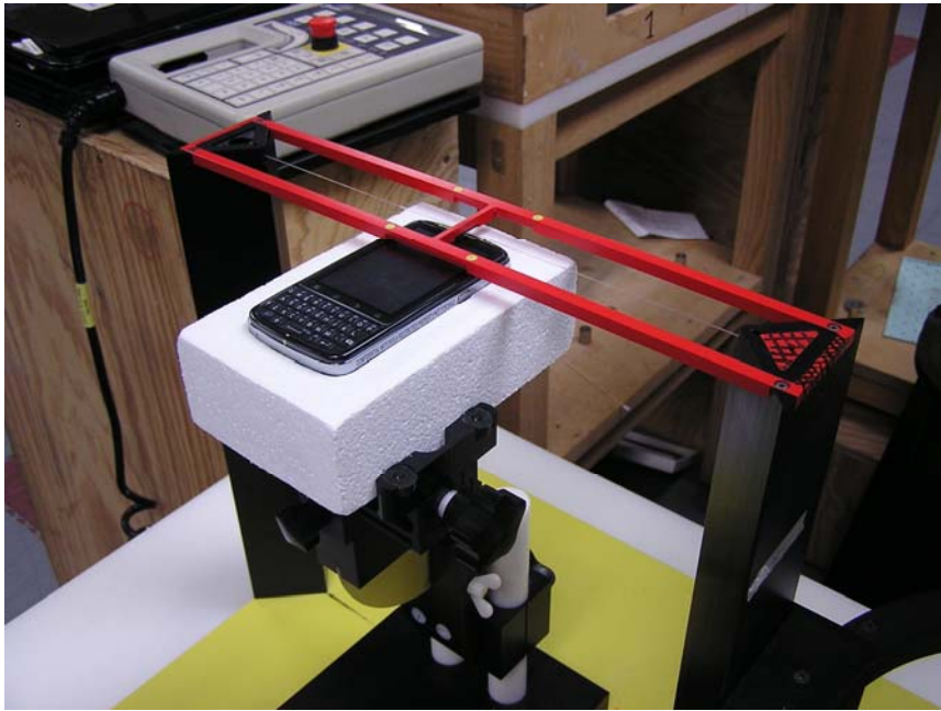
Figure 2. Positioning and Measurement for RF Emissions
