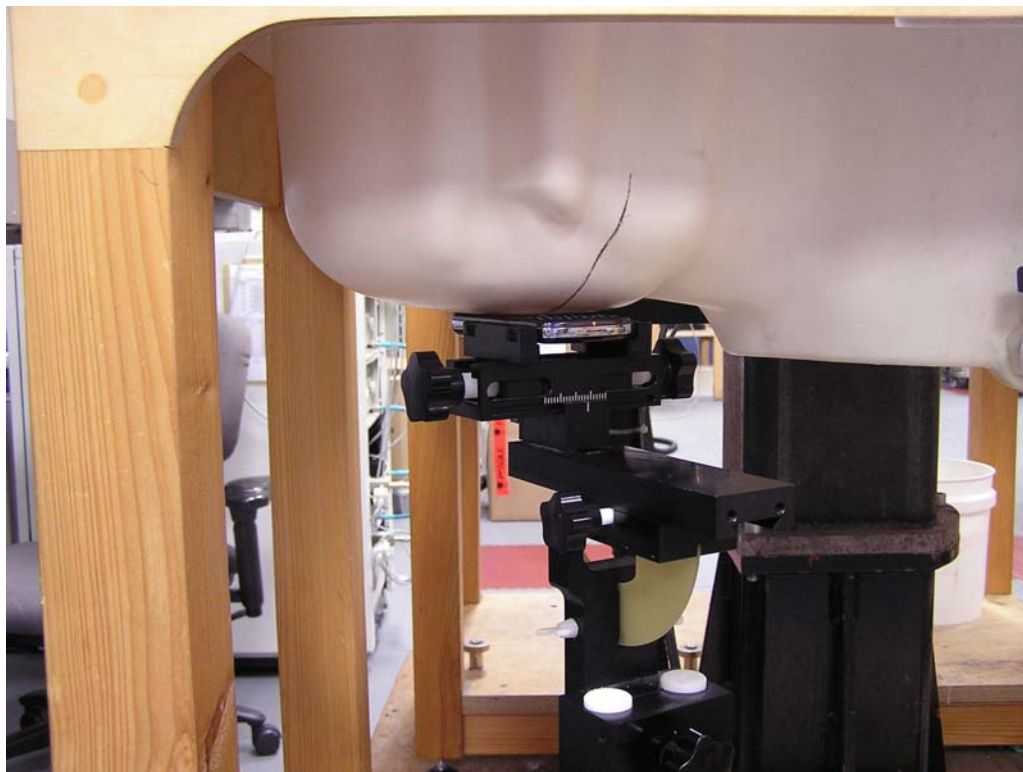
Figure 3: Cheek Position, Front of Head of Phantom
