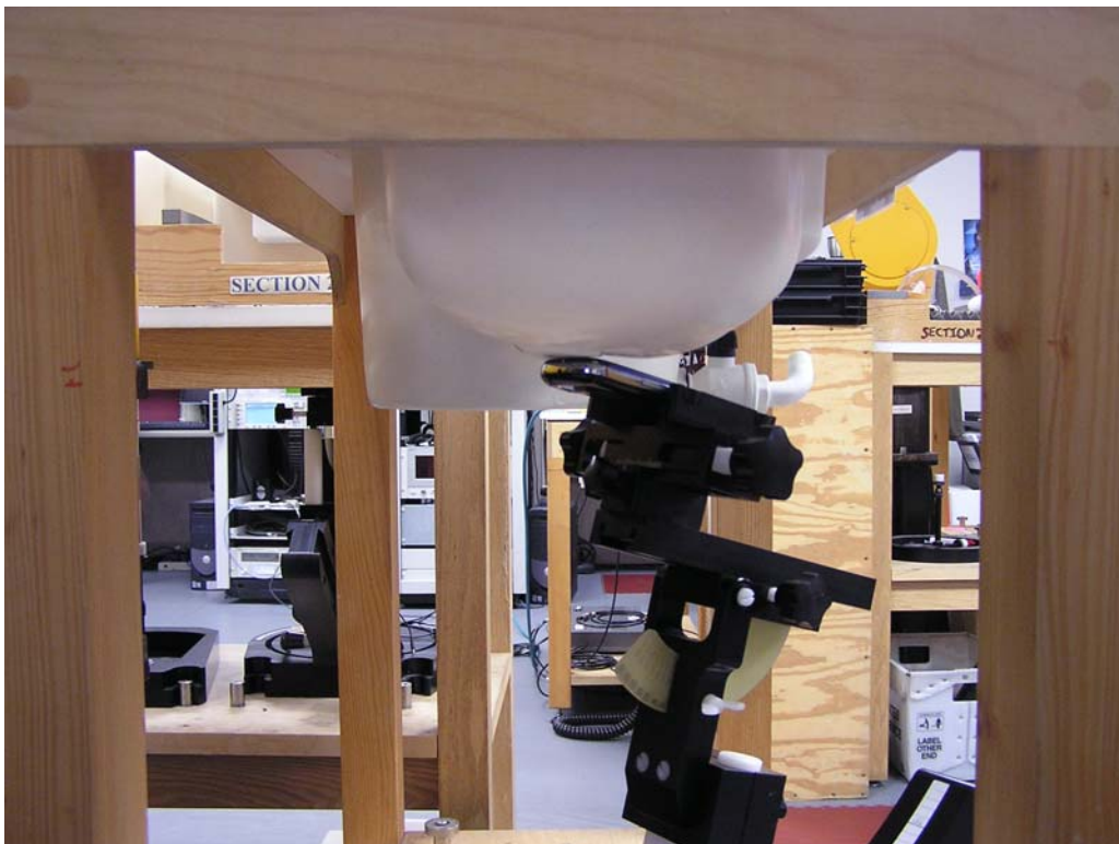
Figure 6: Tilt Position, Top of Head of Phantom
