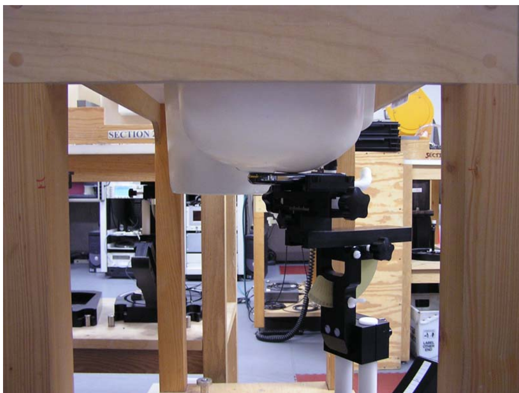
Figure 4: Cheek Position, Top of Head of Phantom
