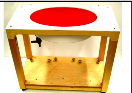
Fig 5.10 Photo of ELI4 Phantom
