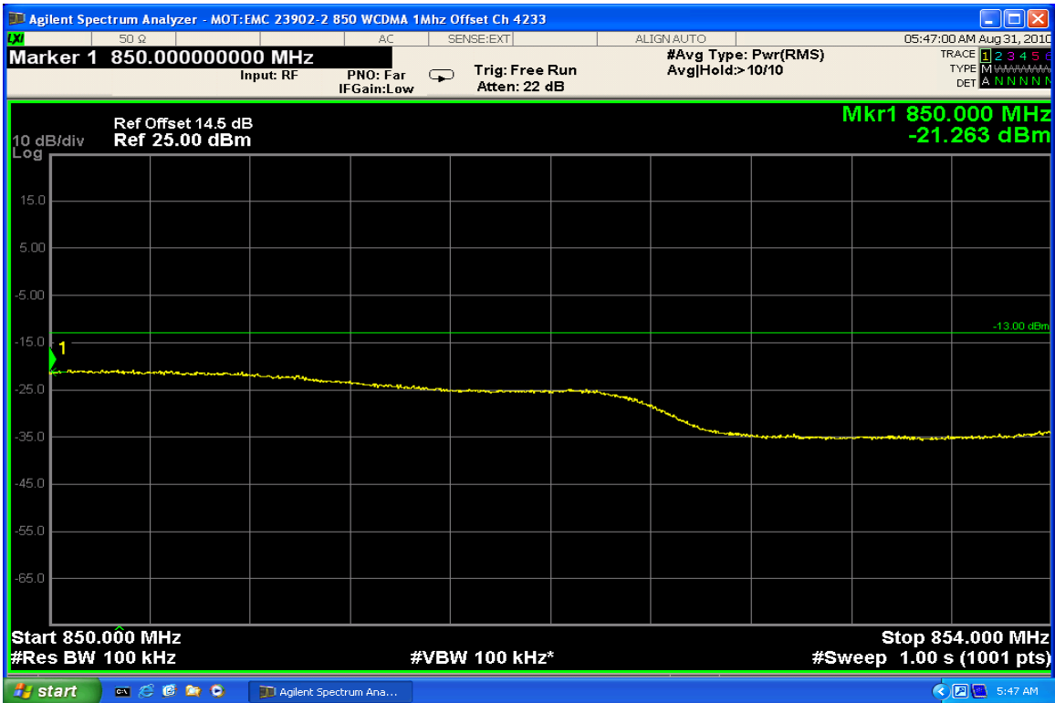
850 WCDMA Conducted Spurious Emissions (Upper adjacent 1 MHz band)
