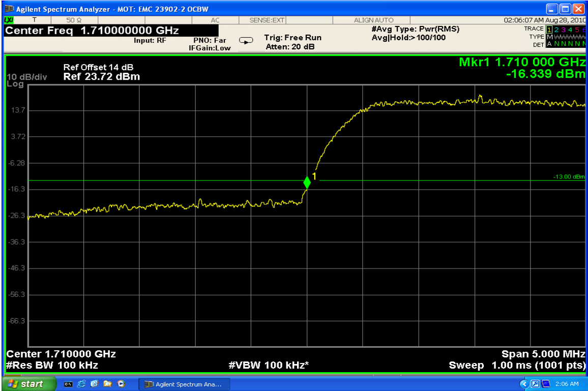
WCDMA 1700 – Lower Band Edge – Channel 1312 (1712.4 MHz)
