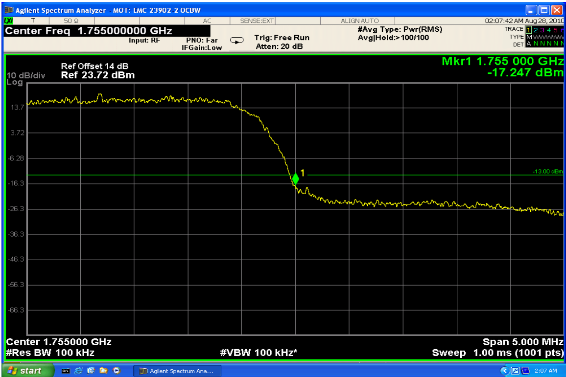
WCDMA 1700 – Upper Band Edge – Channel 1513 (1752.6 MHz)
