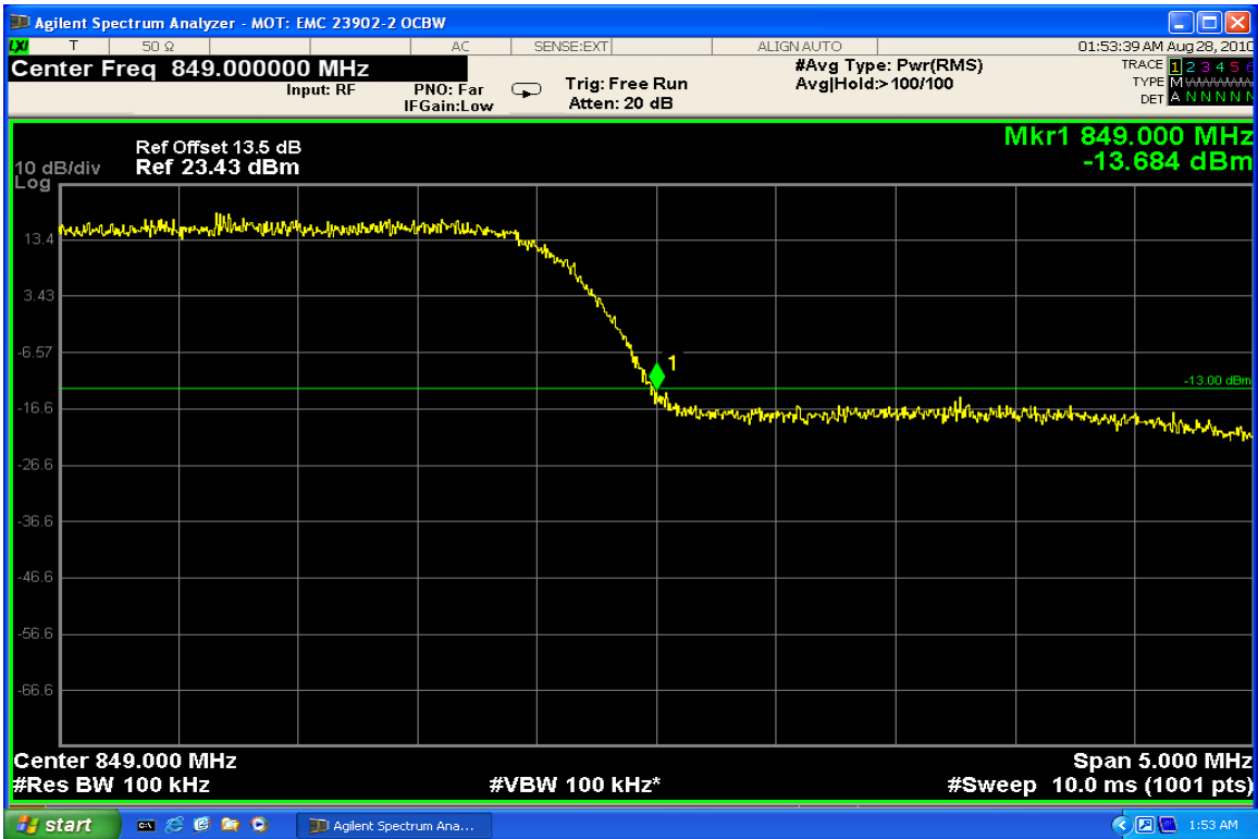
WCDMA 850 – Upper Band Edge – Channel 4233 (846.60 MHz)
