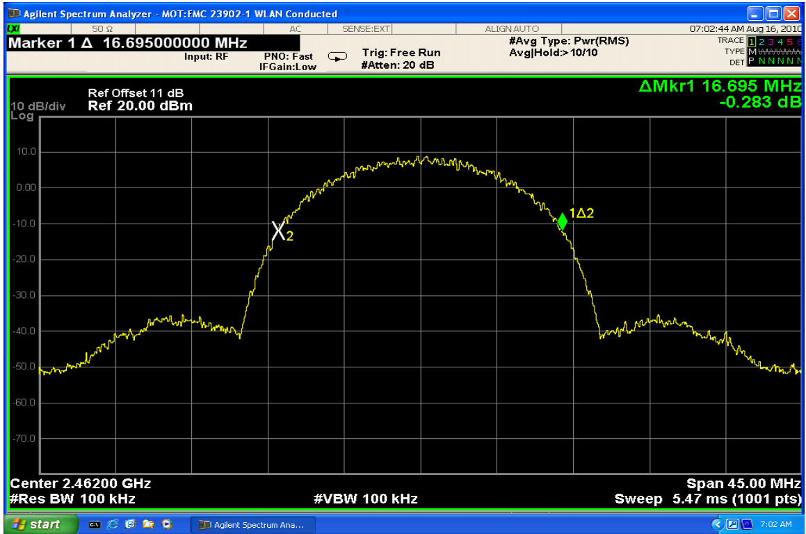
20 dB Bandwidth Channel 11 @ 11Mbps
