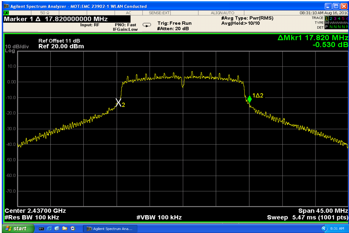
dB Bandwidth Channel 6 @ 9Mbps
