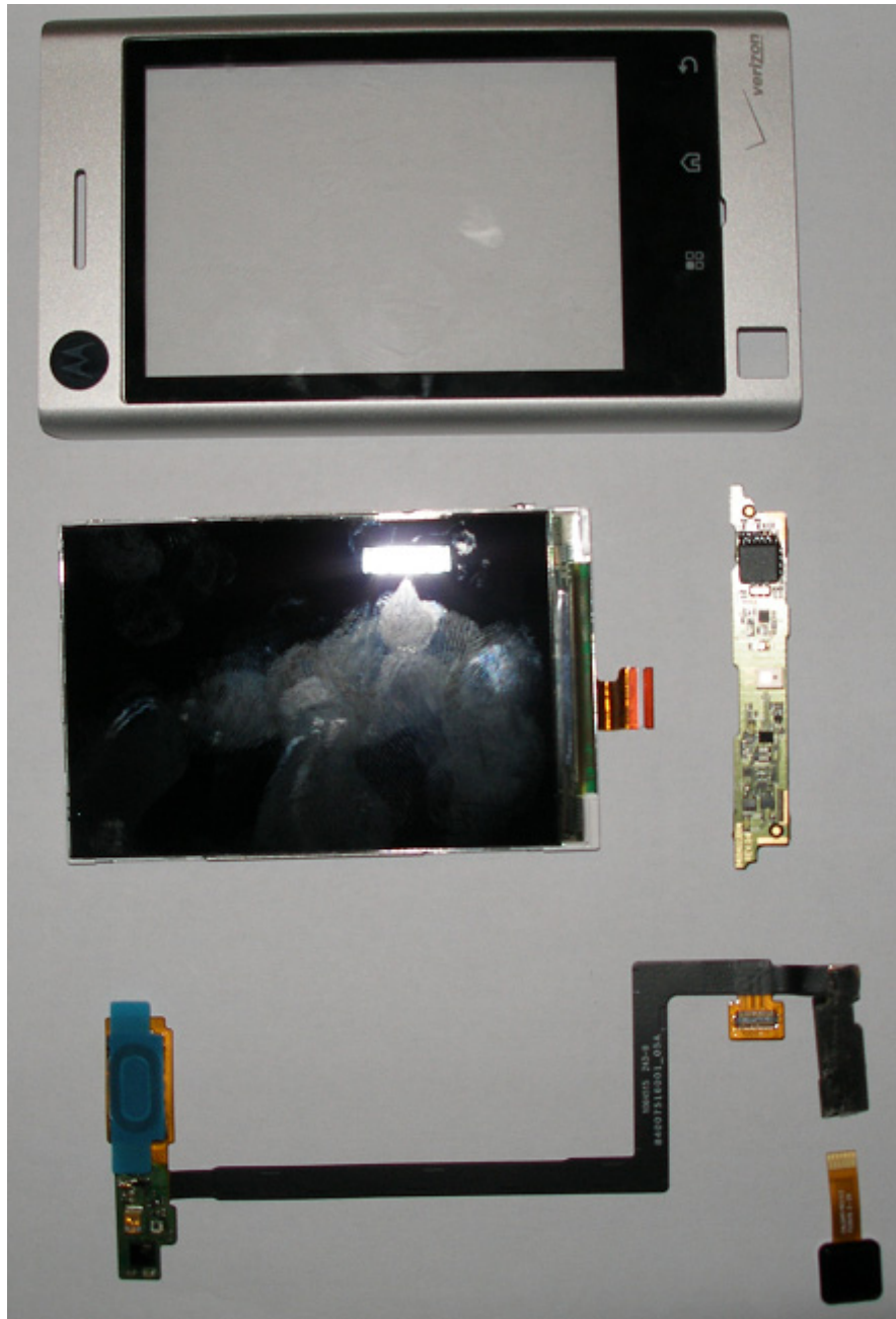
Slide Disassembled Front view
