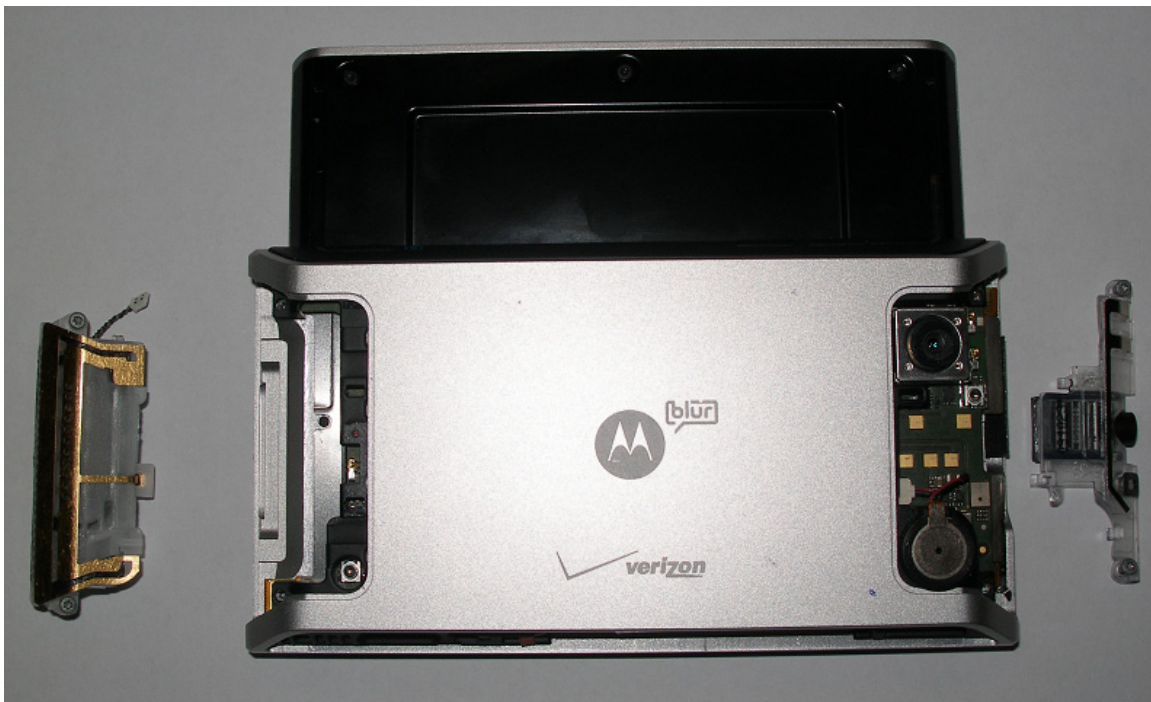
Rear View Antenna carriers off
