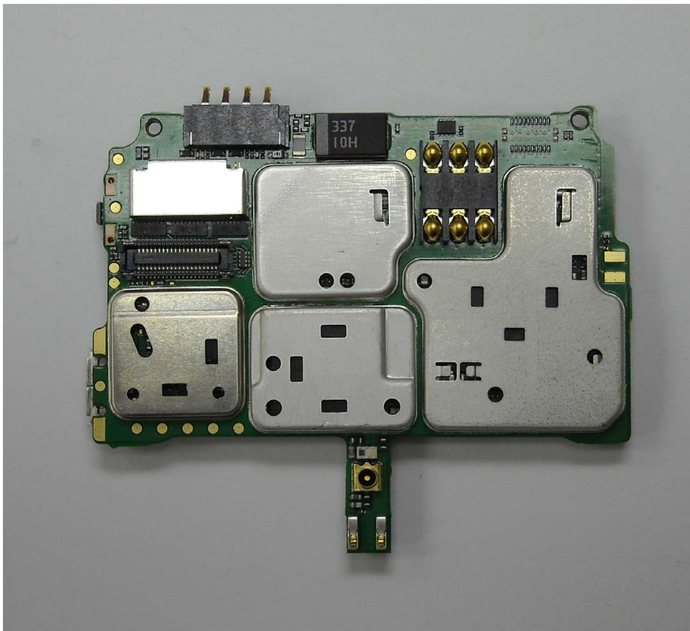
Photograph 9-3: Back side view of PC Board, Shields in place.
