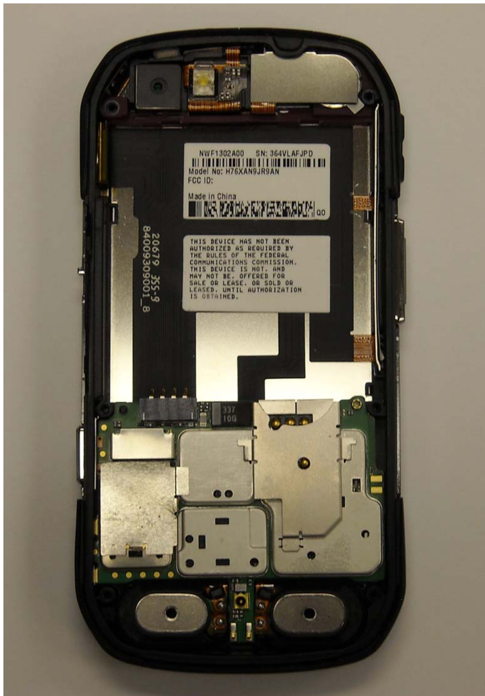
Photograph 9-1: Back side view of radio, back housing removed, showing PC Board.
