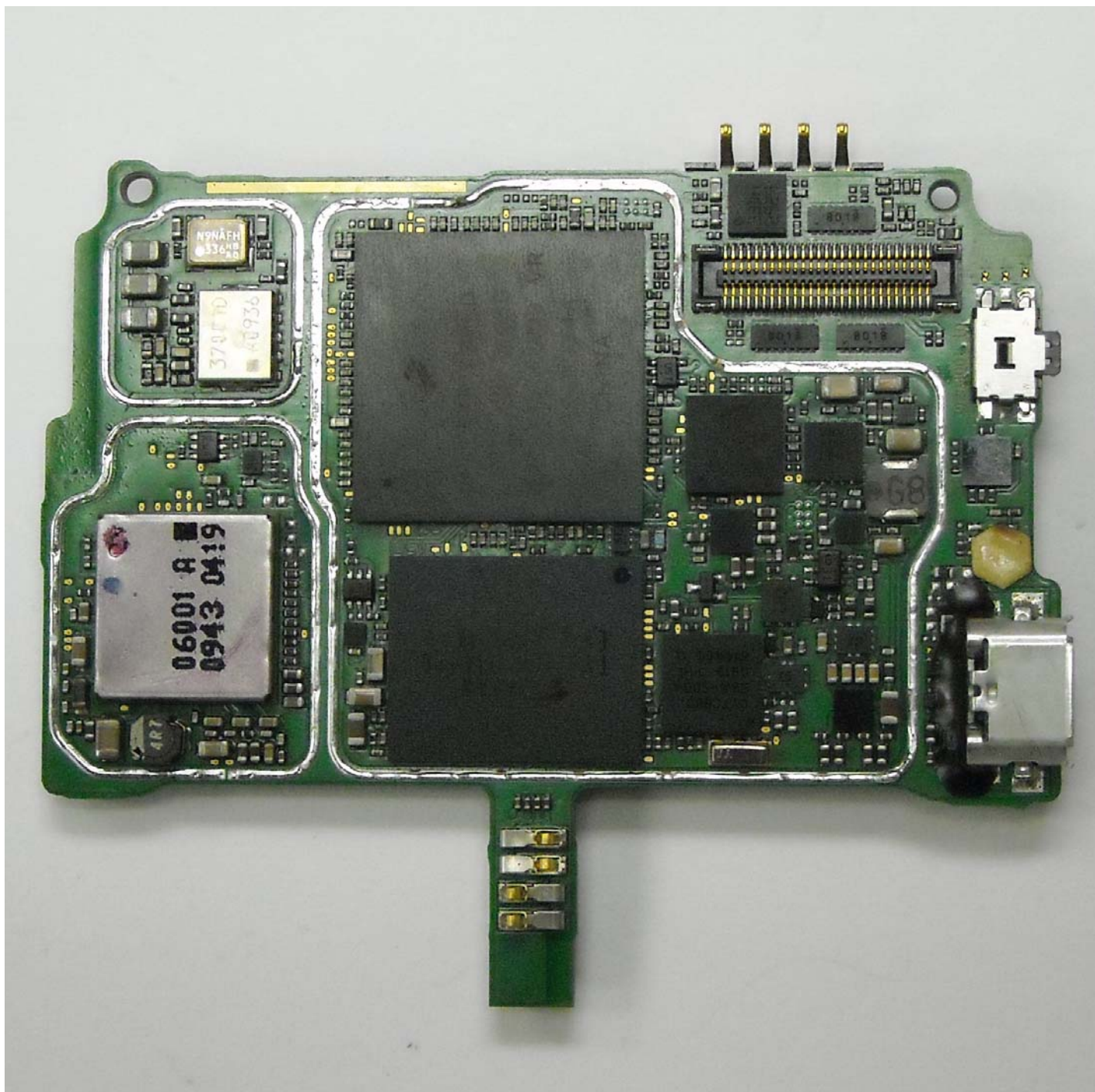
Photograph 9-6: Front side view of PC Board, Shields removed.
