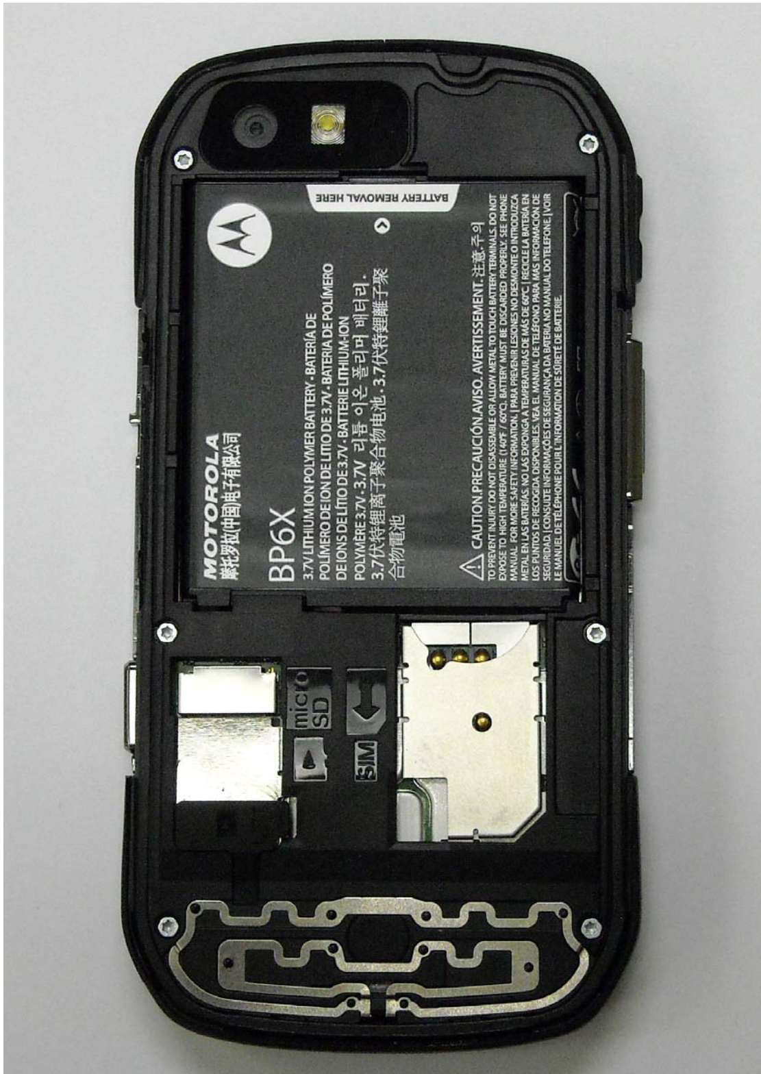
Photograph 9-2: Back side view of radio, Battery Cover removed, showing Main Antenna.
