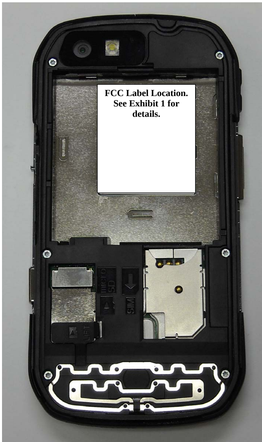
Figure 3-7. Interior Compartment of radio
