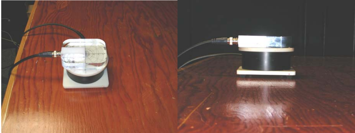
Figure 6-1 – Probe coil being calibrated with TMFS
