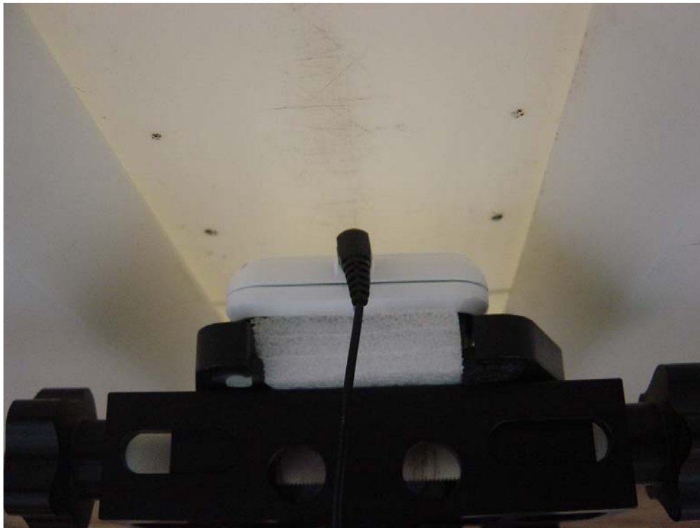
Figure 9: Phone Against the Flat Phantom
