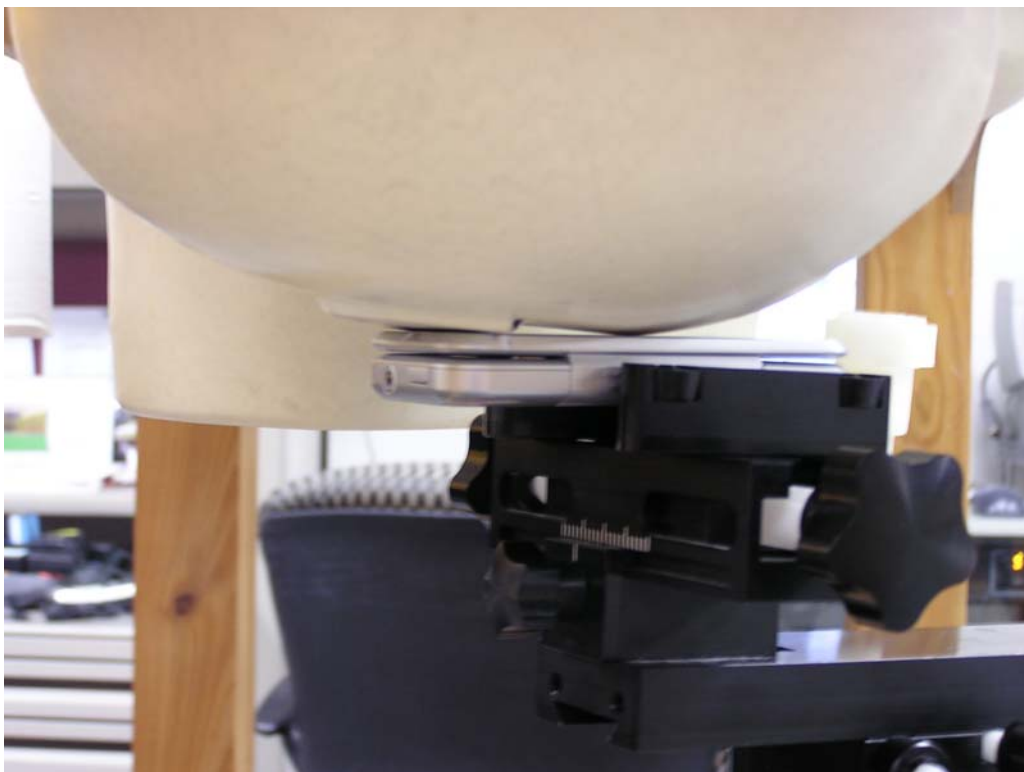
Figure 4: Cheek Position, Top of SAM Phantom
