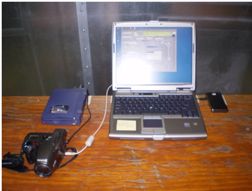
AC Line Conducted Emissions – Computer Peripheral
