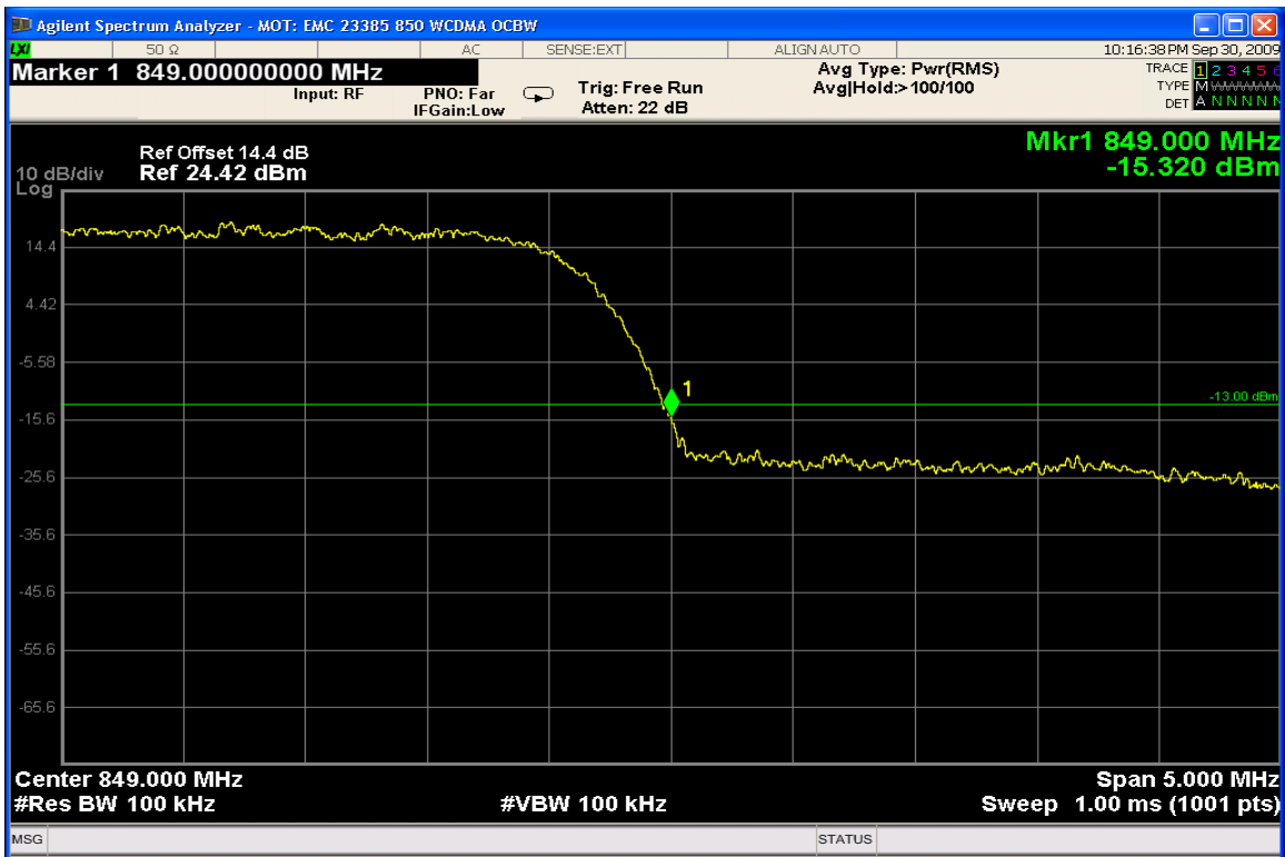
WCDMA 850 – Upper Band Edge – Channel 4233 (846.60 MHz)
