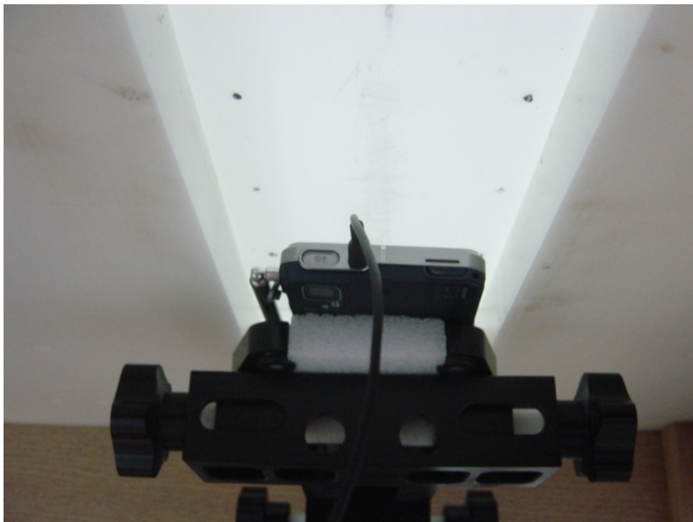
Figure 6: Back of Phone Against the Flat Phantom with DMB Antenna Position 1 (15mm distance)
