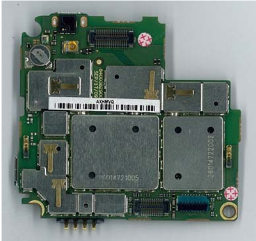
Main Board Top With Shields
