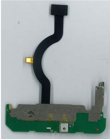
Audio Board Top With Shield
