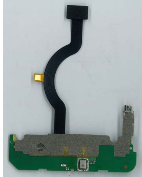
Audio Board Top Without Shield
