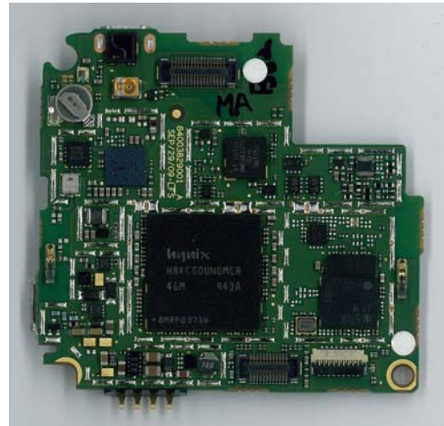
Main Board Top Without Shields
