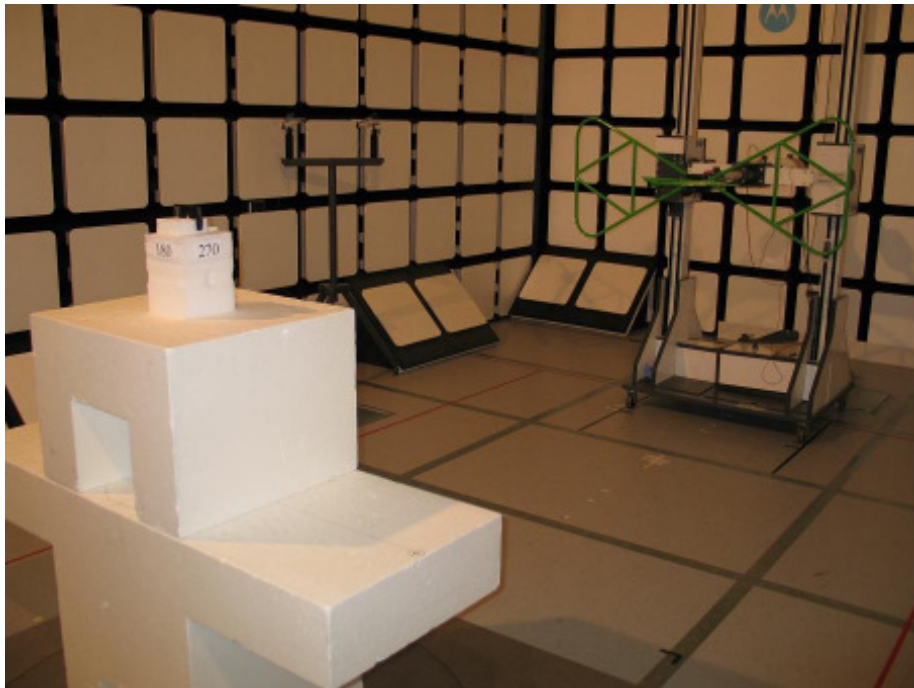
22333-1, IHDP56JX2 setup in semi-anechoic chamber – right view
