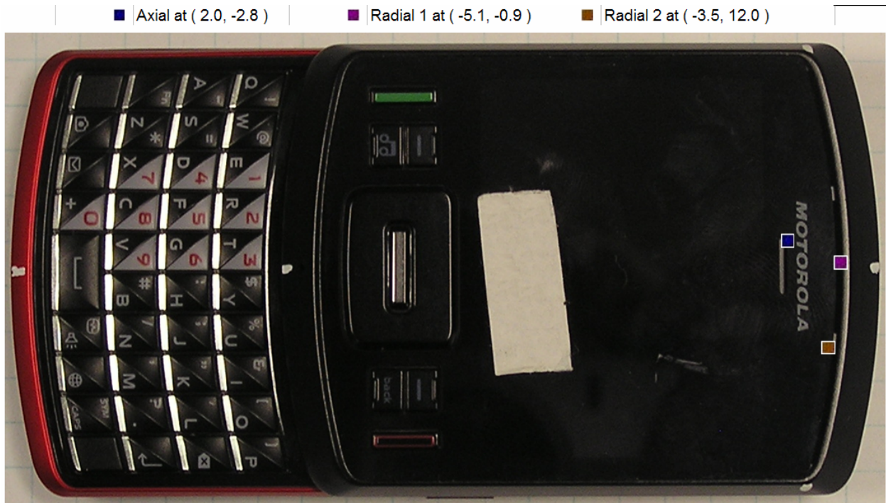
Figure 7. Location of Measured Points for Telecoil measurements
