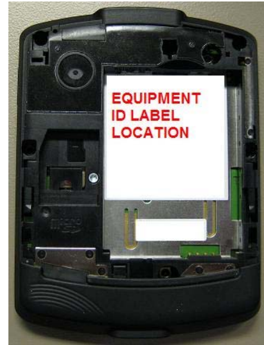
BACK OF PHONE WITH BATTERY COVER REMOVED
