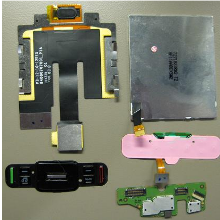
Slider assembly – Flex, LCD, keypad, and PCB.
