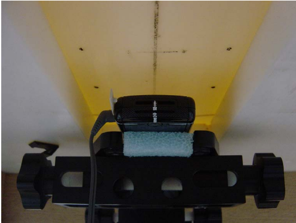
Figure 5: Phone Against the Flat Phantom
