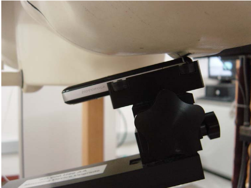
Figure 4: Phone Against the Head Phantom (15° Tilt)
