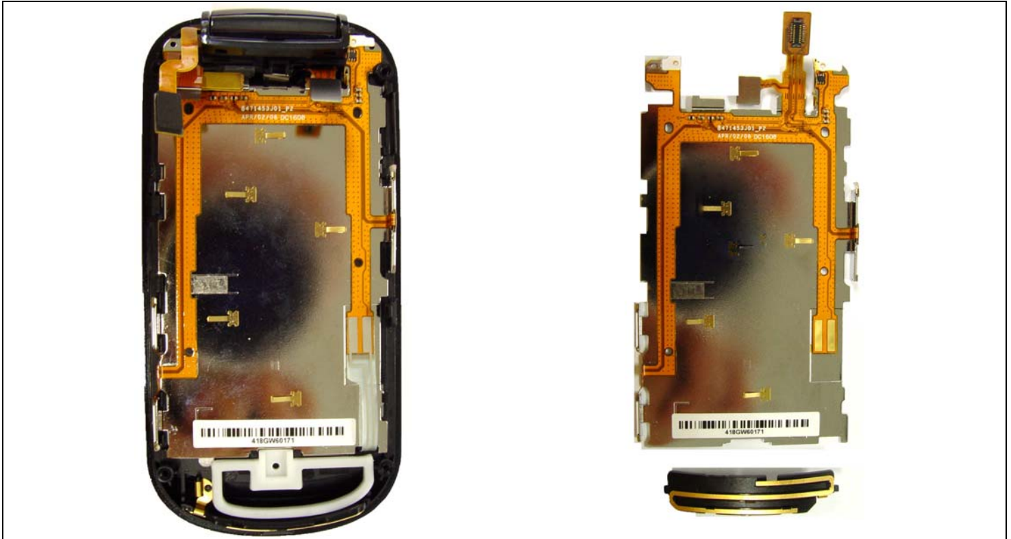
Internal Housing view of Main Front Part
