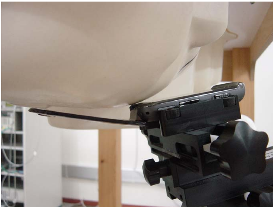
Figure4: Phone Against the Head Phantom (Cheek Touch)
