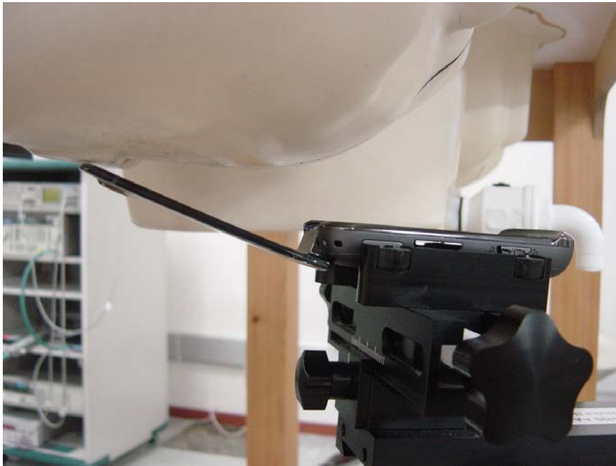
Figure5: Phone Against the Head Phantom (15° Tilt)
